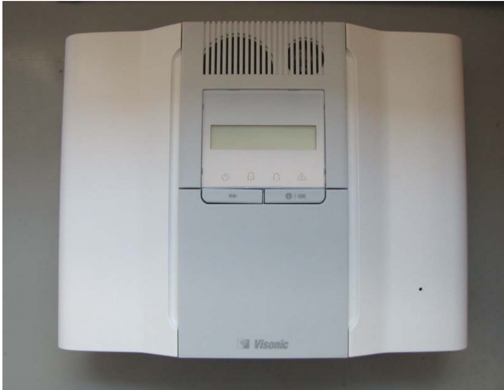
Photograph No.1 PowerMaxComplete control panel general view
