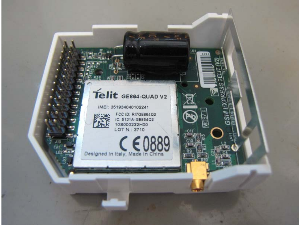
Photograph No.16 GSM modem rear side view
