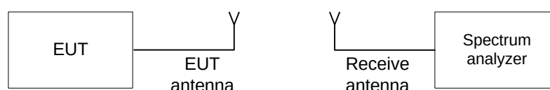
Figure 7.7.1 Band edge emission test setup
