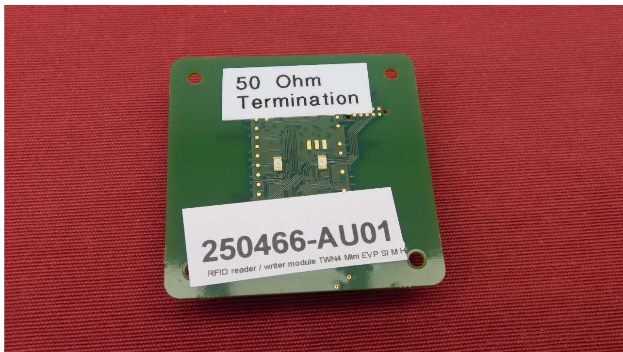
Picture 5: Top view of EUT, with 50 \Omega termination
