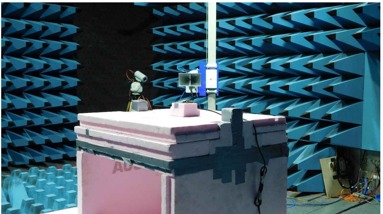
Picture 6: FS-SAC, radiated emission test 1 GHz – 2 GHz (rear view)
