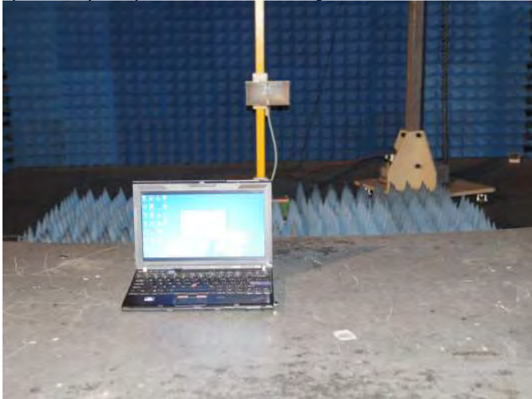
Photograph 8: Set-up for Spurious Emissions of Remote, 18GHz – 25GHz
