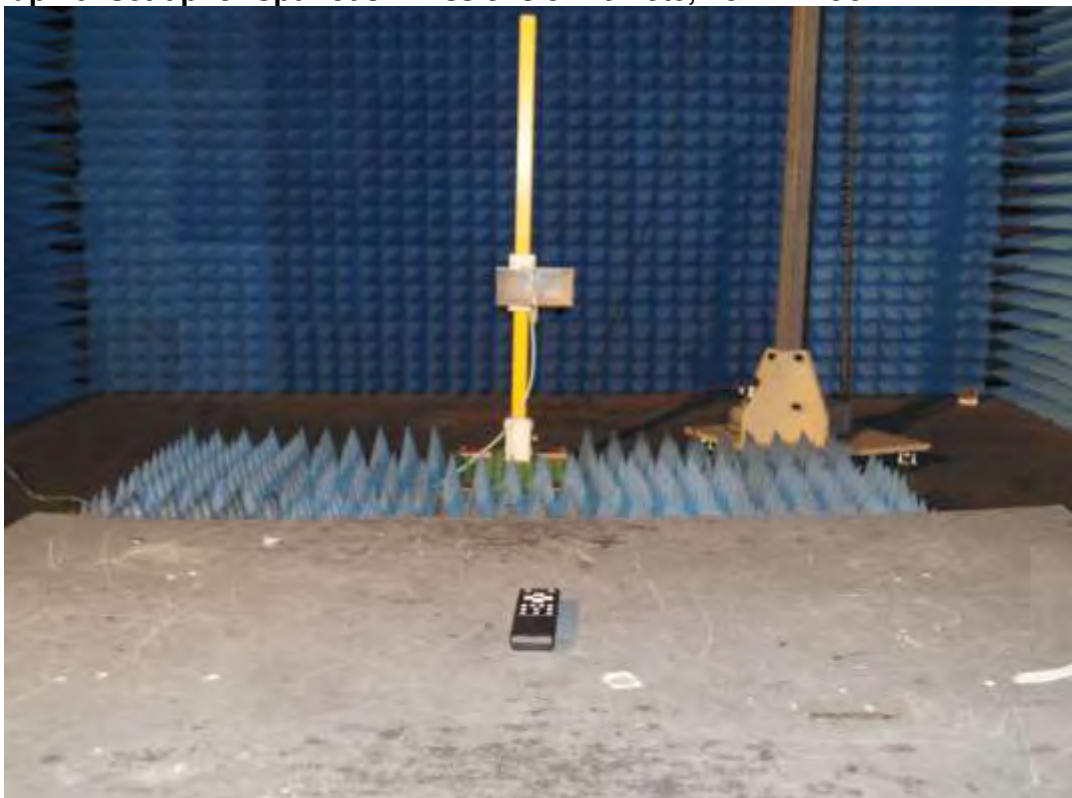
Photograph 6: Set-up for Spurious Emissions of Remote, 1GHz – 18GHz
