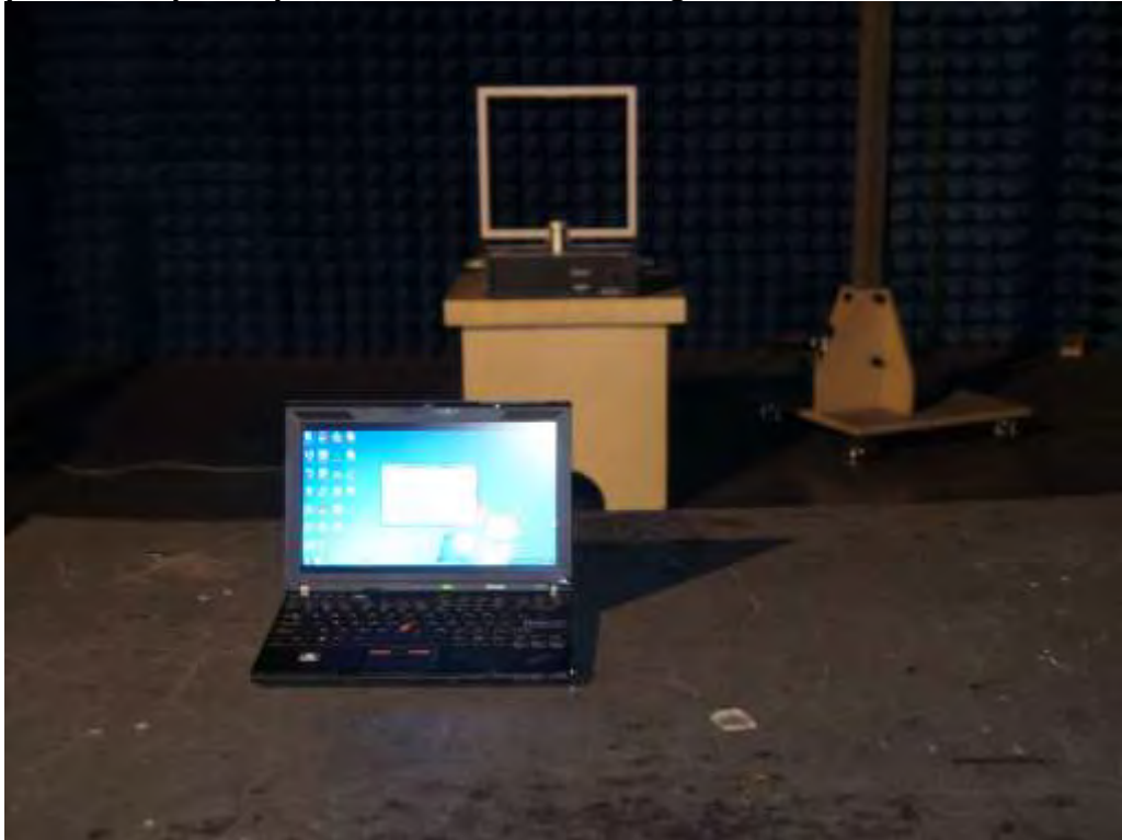
Photograph 4: Set-up for Spurious Emissions of Remote, 30MHz - 1GHz
