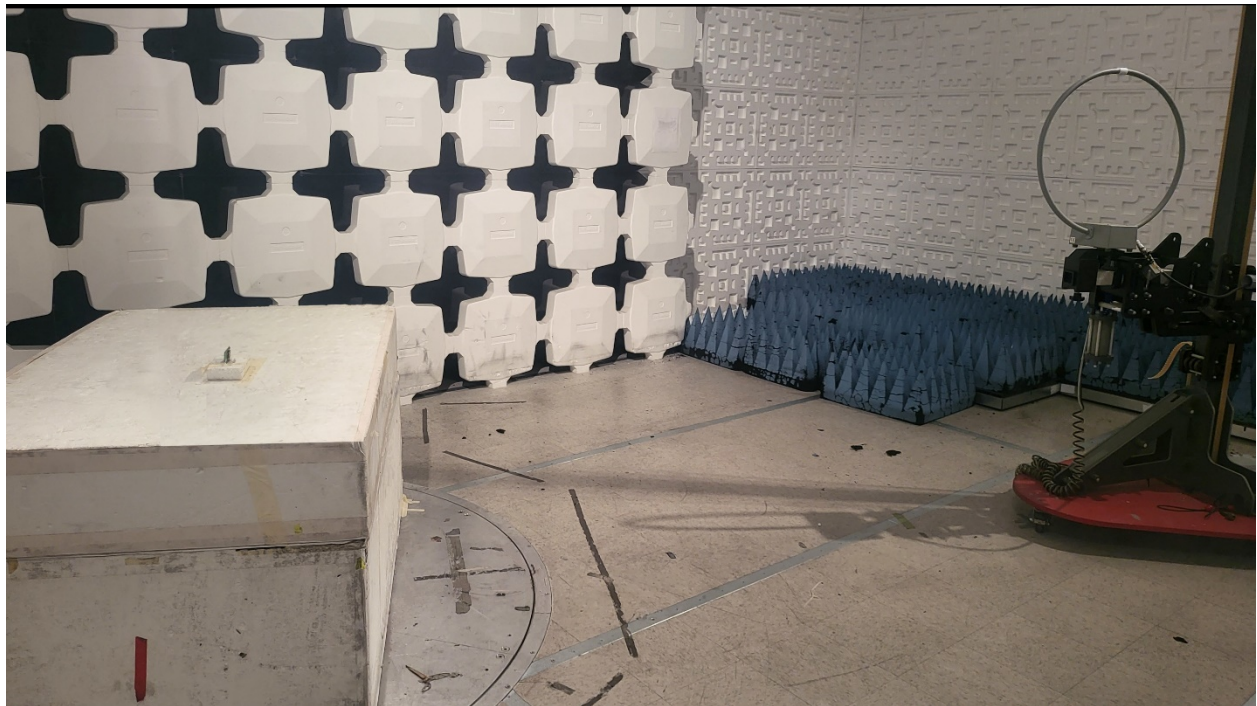
Figure 2. Test Configuration below 30 MHz using Loop Antenna
