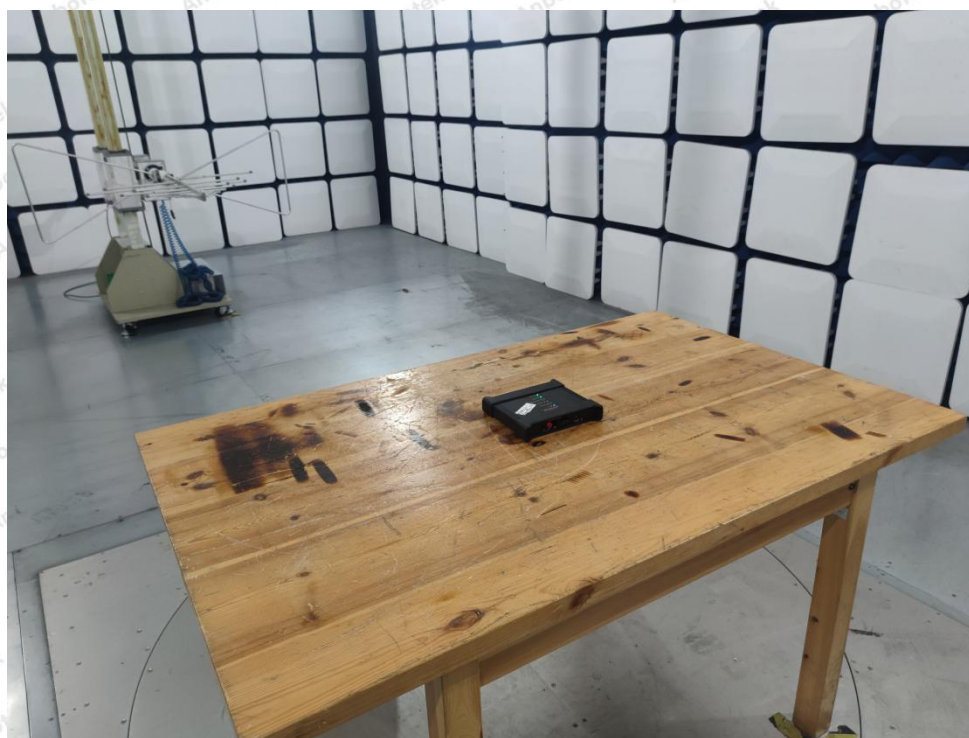
Photo of Radiation Emission Test
