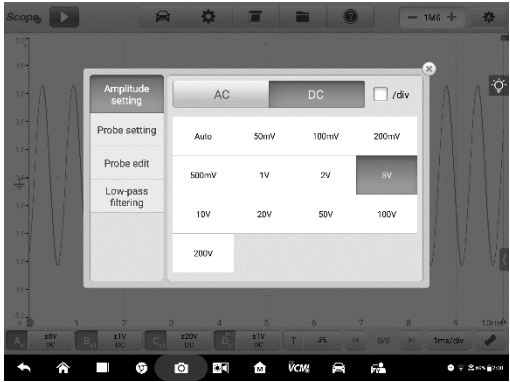
Figure 8-37 Channel Setting Dialog Box Screen
