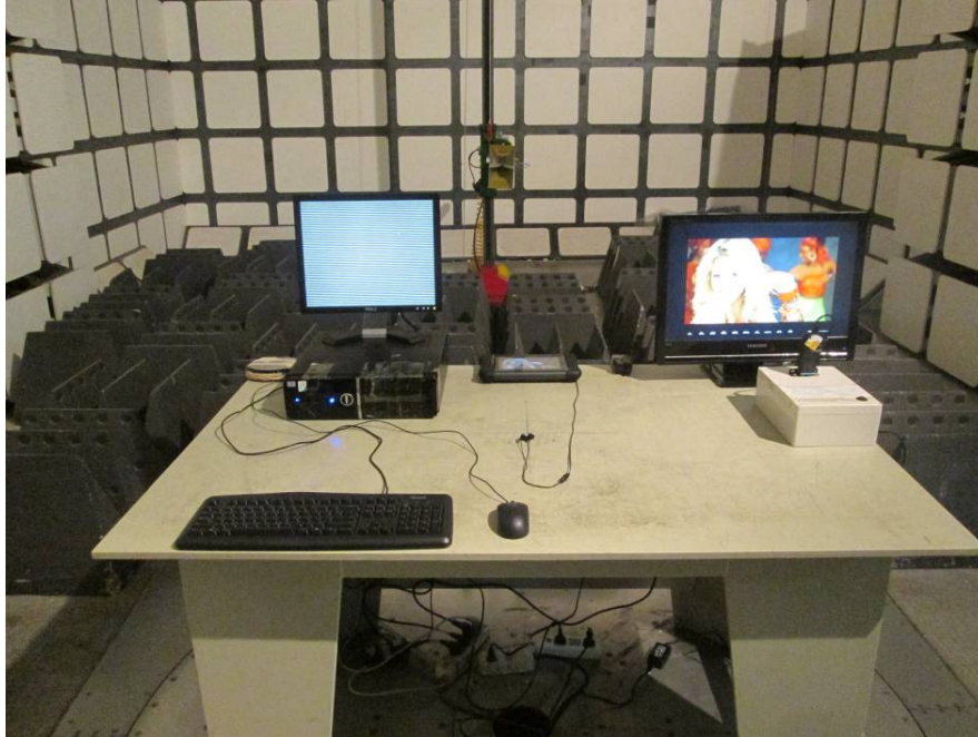
Radiated Emissions – Front View (Above 1 GHz)
