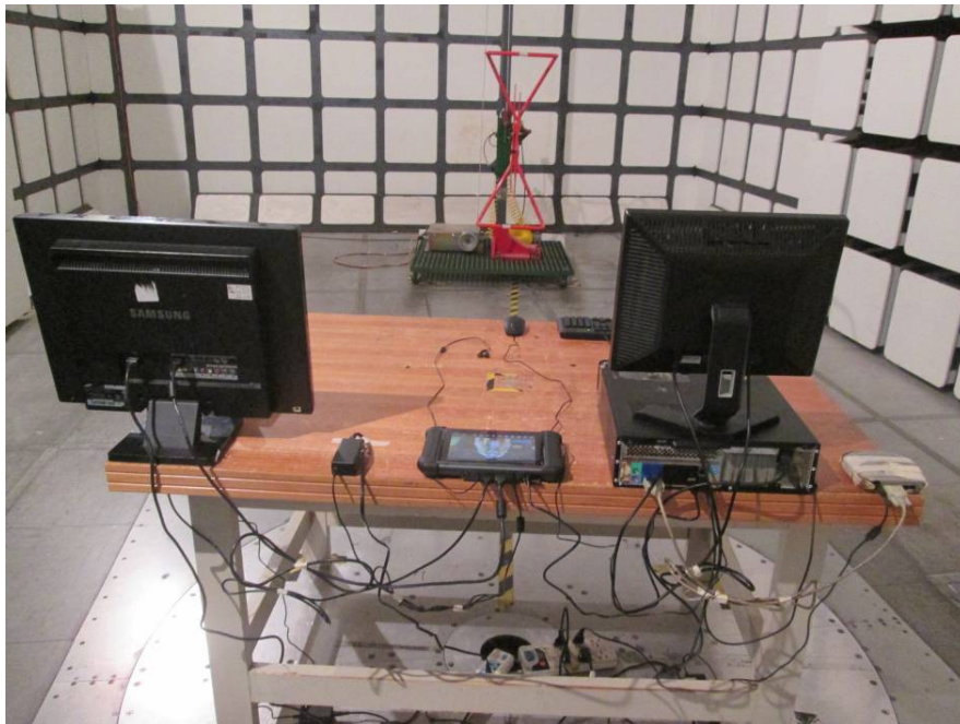
Radiated Emissions – Rear View (Below 1 GHz)
