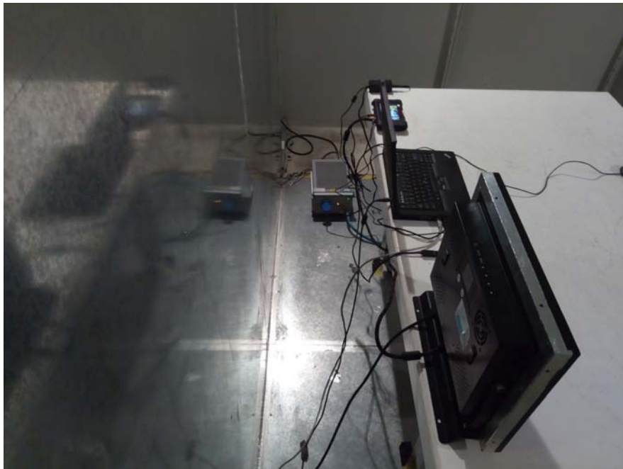
Conducted Emissions - Side View
