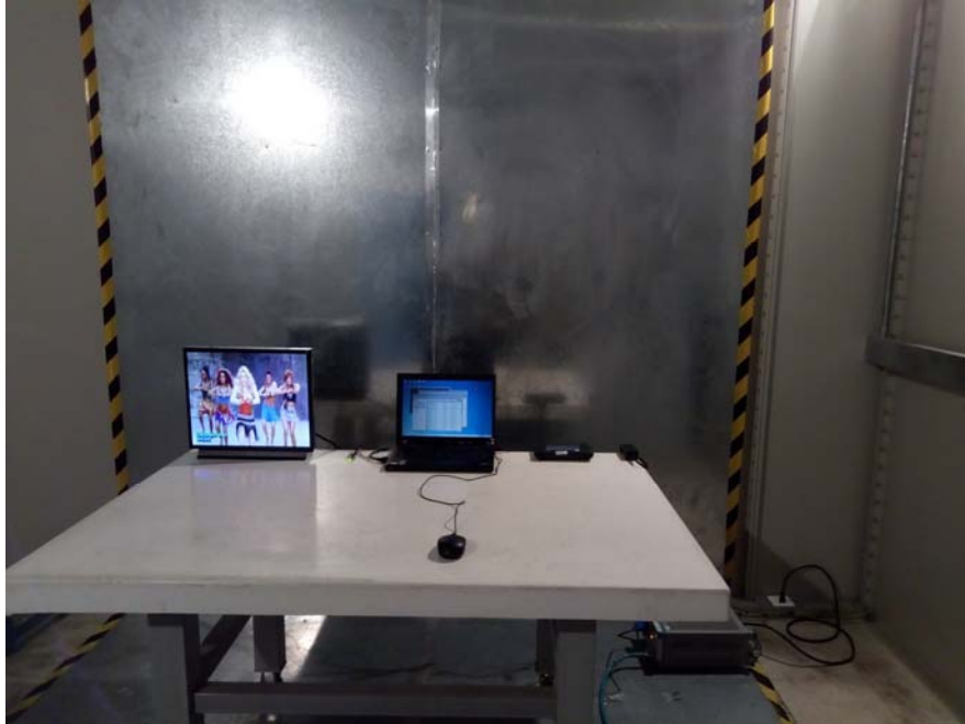
Conducted Emissions - Front View
