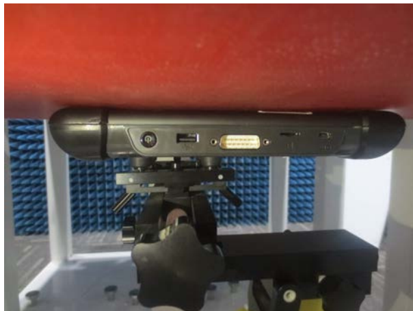
Front with Phantom 0 mm Gap
