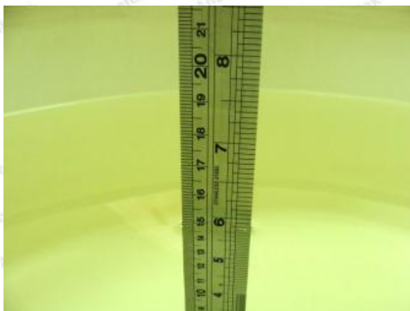
Photo of Liquid Height for Body SAR
