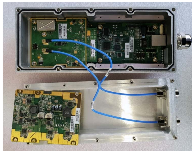
WIN5137-AC Internal view – Without PSU board
