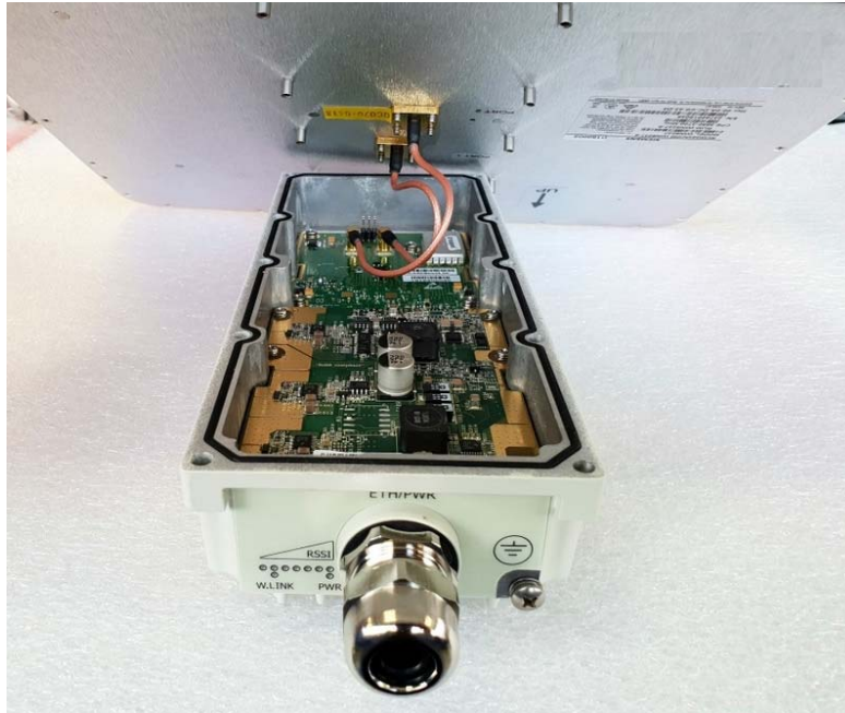
WIN5237 Internal view - Without PSU board
