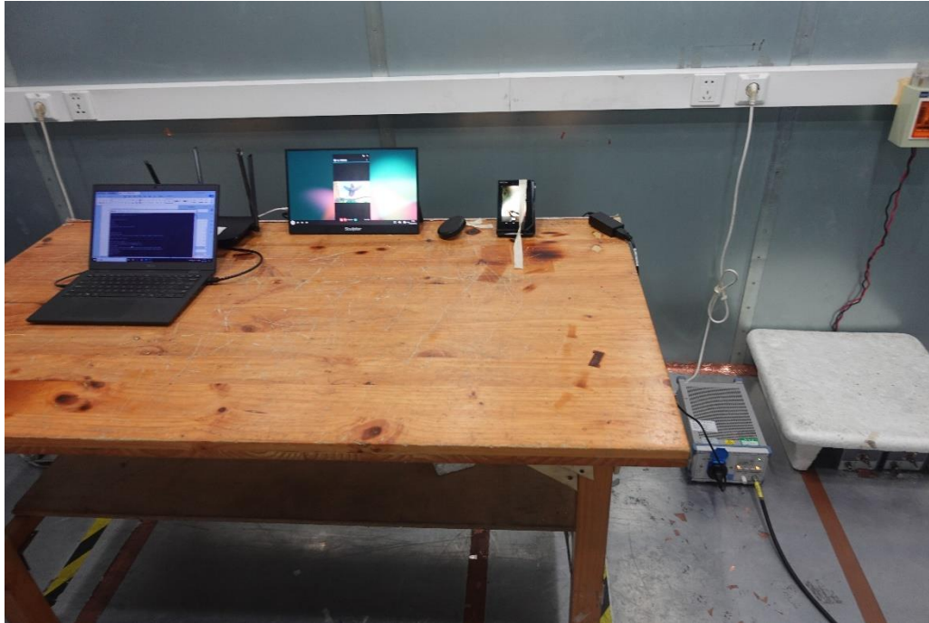
Picture 2 Conducted Emission Test Setup
