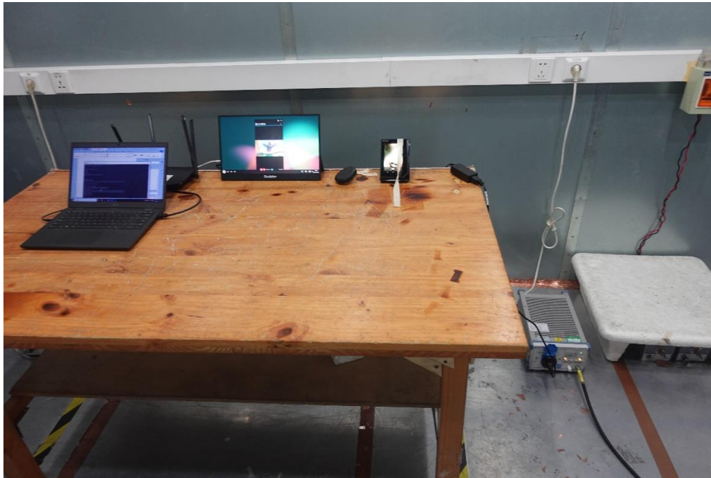
Picture 2: Conducted Emissions Test Setup
