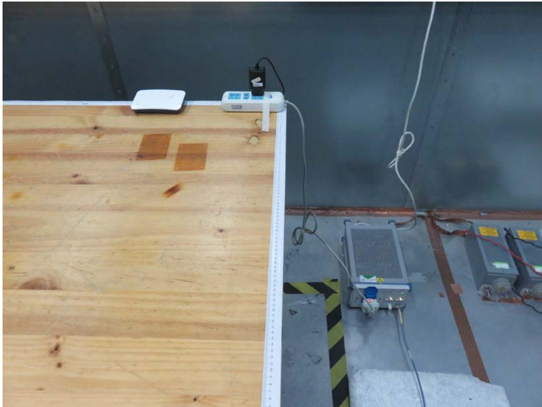
Picture 3 Conducted Emission Test Setup
