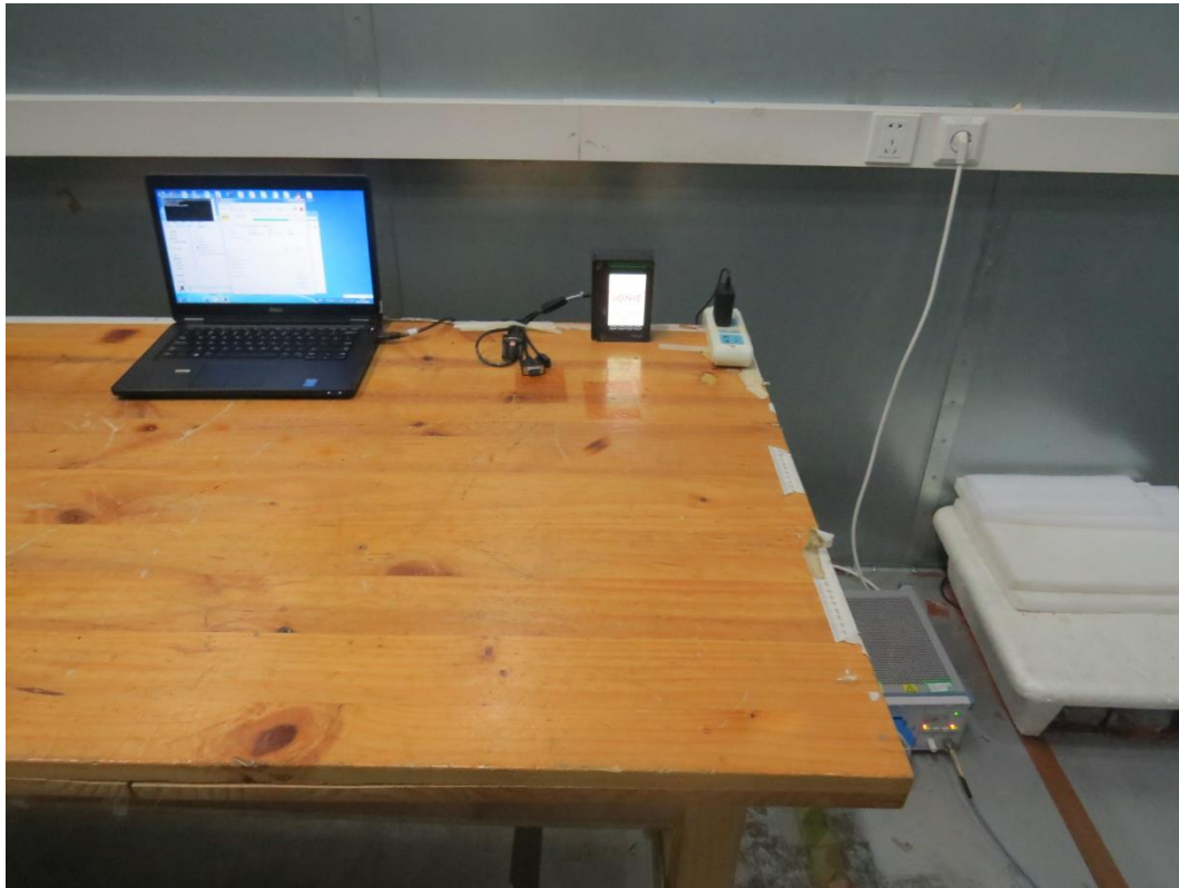
Picture 3 Conducted Emission Test Setup
