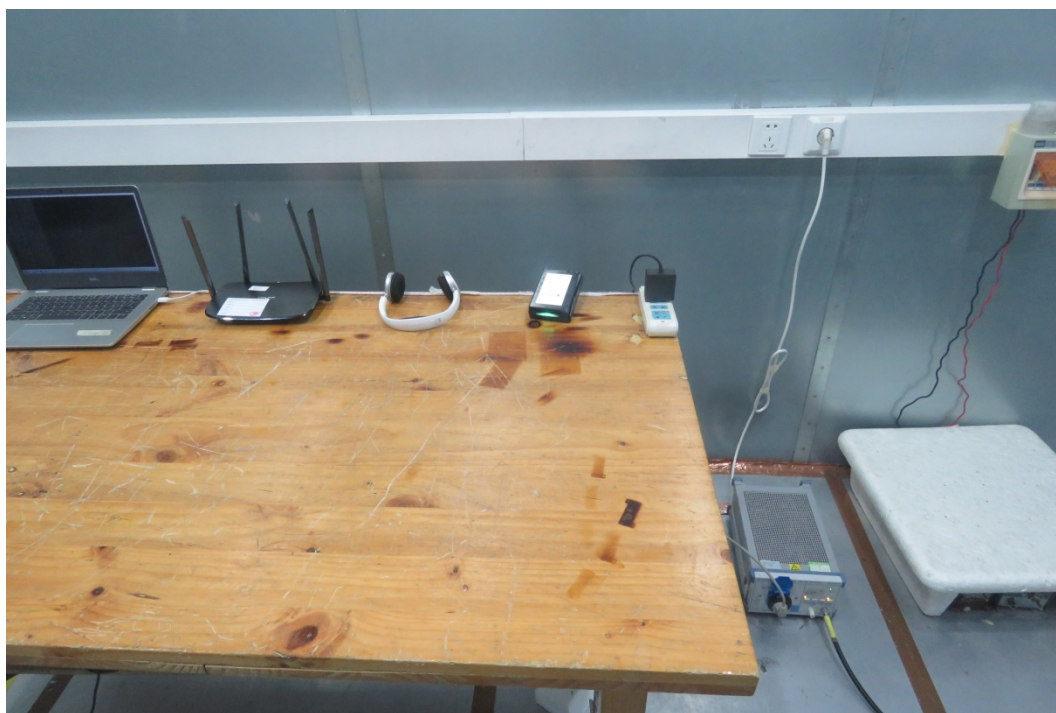
Picture 2: Conducted Emissions Test Setup
