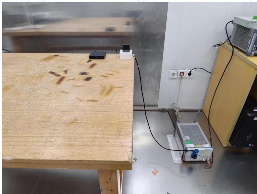
Photo of Setup for Radiated Emission (30MHz~1GHz)
