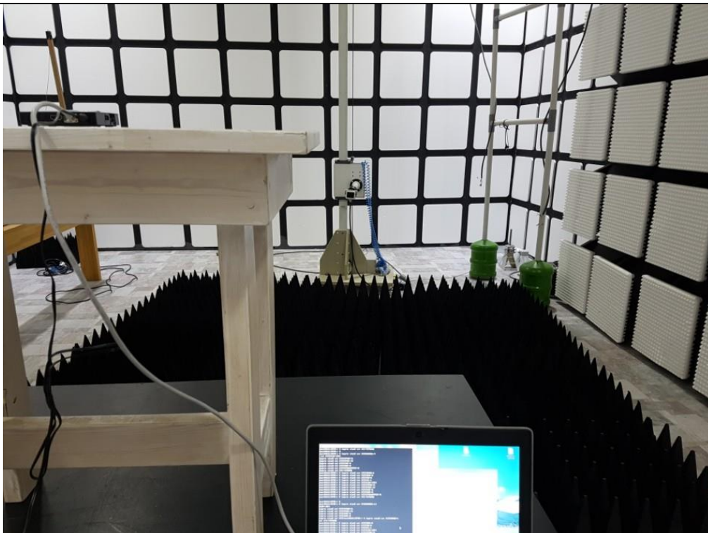
Radiated Test (Above 1G)
