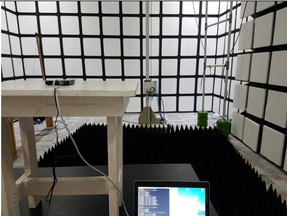
Radiated Test (Above 1G)
