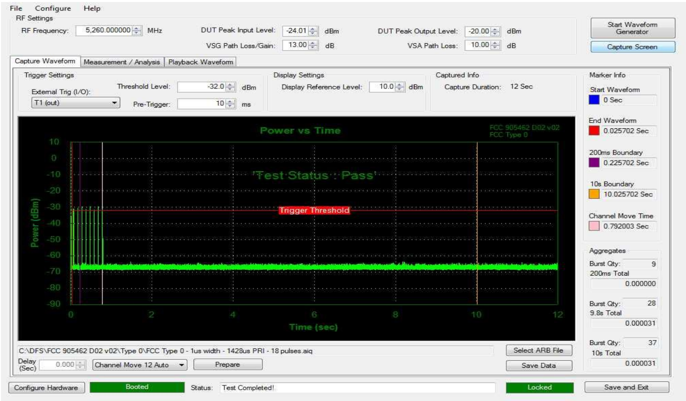
Figure 8.6-1: Channel closing transmission and move time
