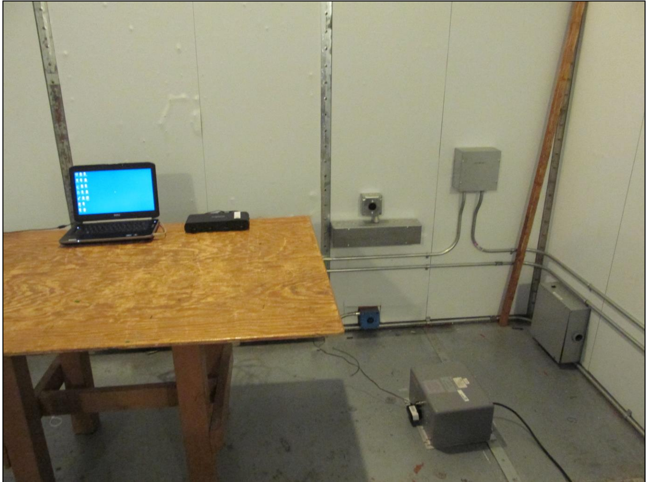
Photograph 2. Conducted Emissions, Test Setup
