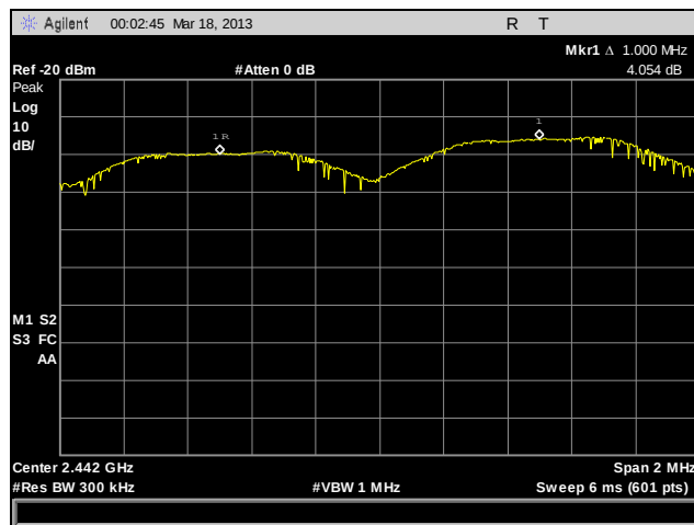
Plot 49. Channel Separation, Mid Channel, Radio 4
