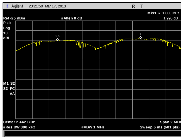
Plot 46. Channel Separation, Mid Channel, Radio 3
