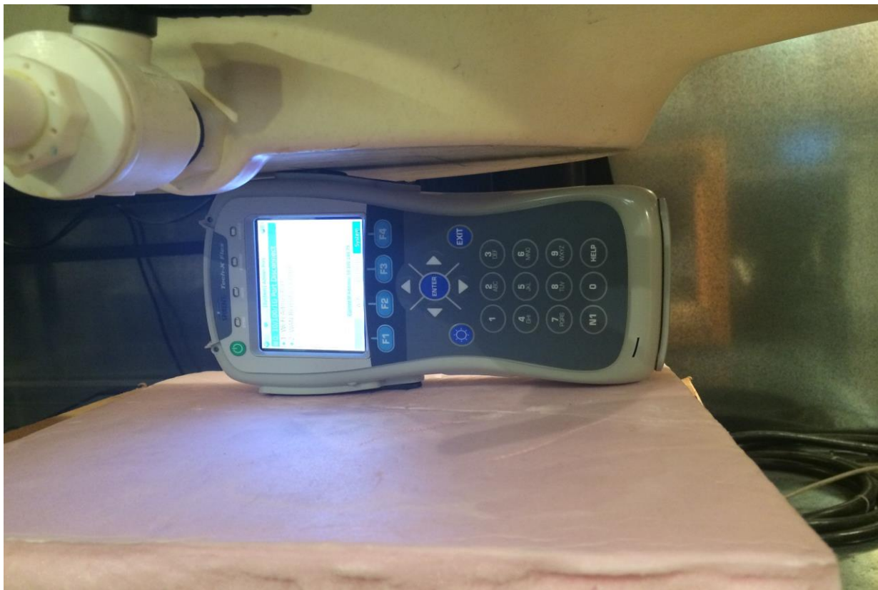
Photograph 1. EUT Right Edge/Antenna, Side against Phantom
