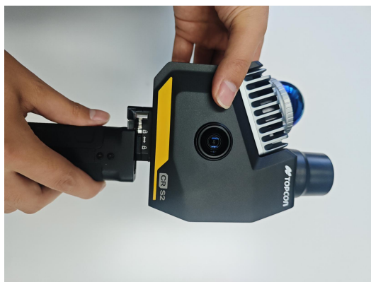
② Open the locking handle, align the battery with the groove at the bottom of the device, and slide it in.
