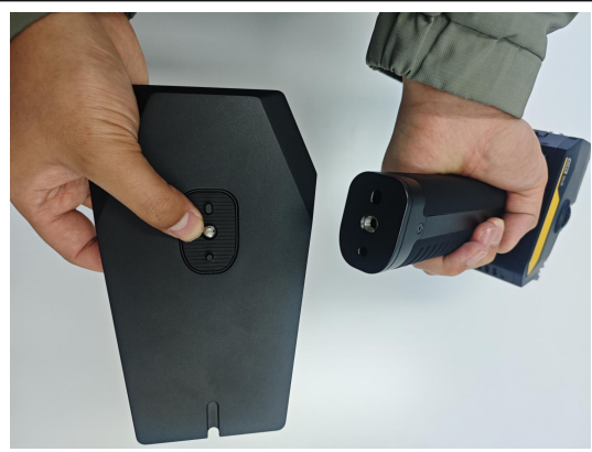
④ Align the base stand with the battery ground hole.
