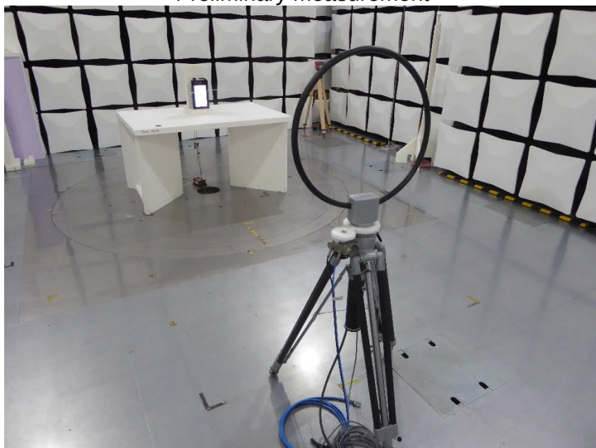
EUT Position 2 – standing / Antenna Position 2 – perpendicular Test setup semi-anechoic chamber M276 Preliminary measurement
