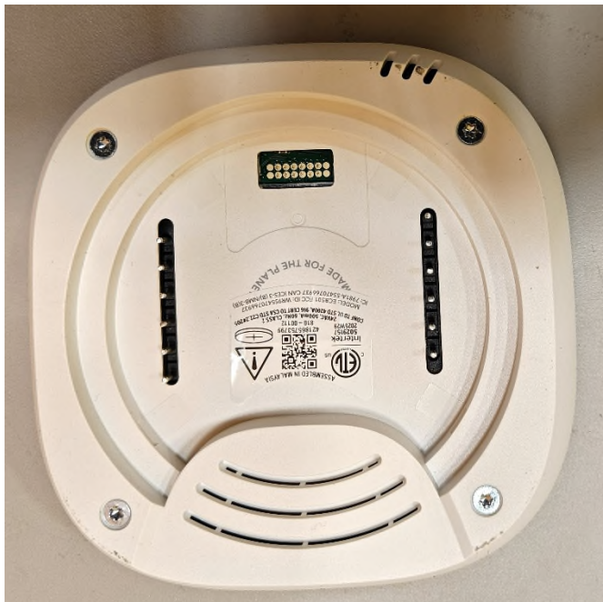
Figure 9 – ECB501: Back view with I/O ports
