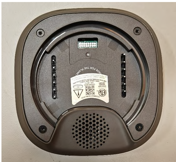
Figure 6 – ECB601 (PLC variant): Back view with I/O ports
