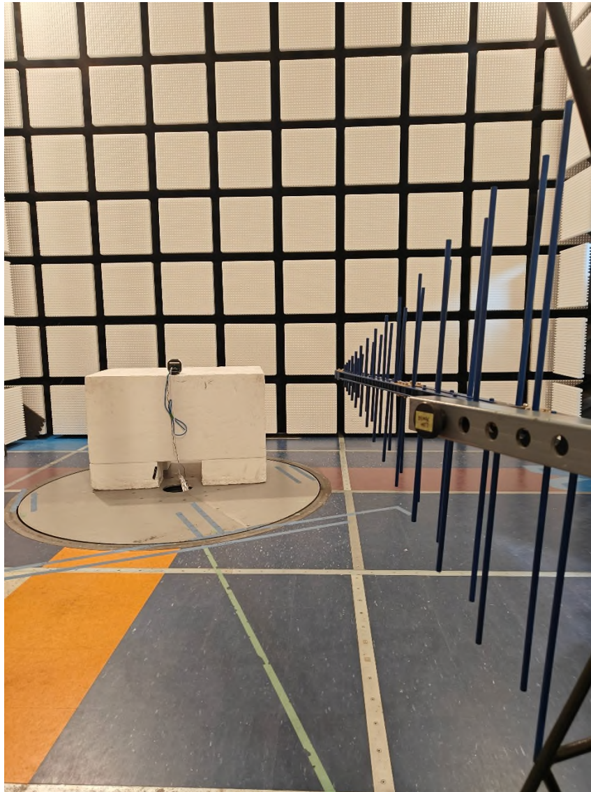
Figure 3 – Radiated Emissions Setup 30MHz – 1GHz
