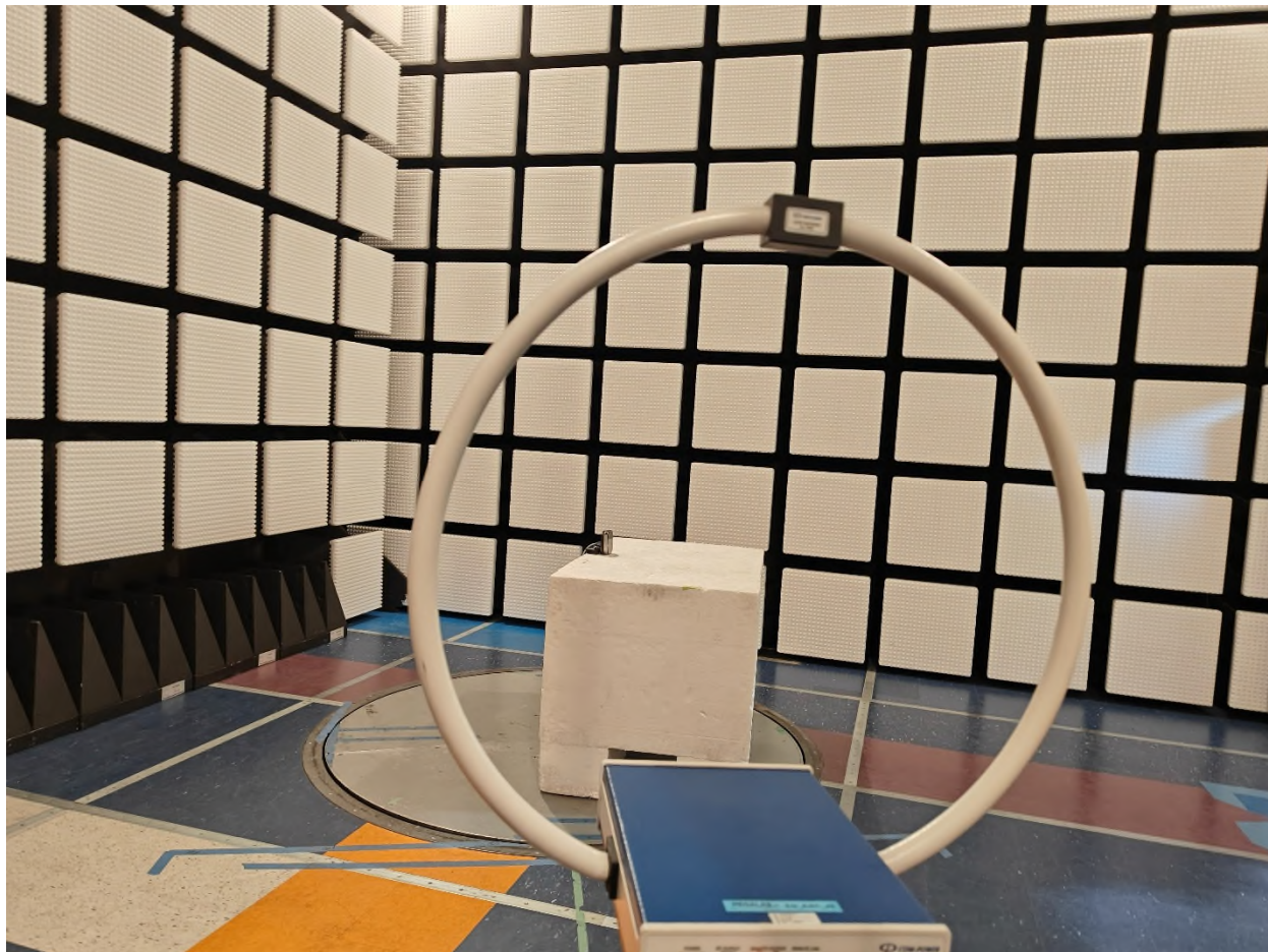
Figure 2 – Radiated Emissions Setup 9kHz – 30MHz
