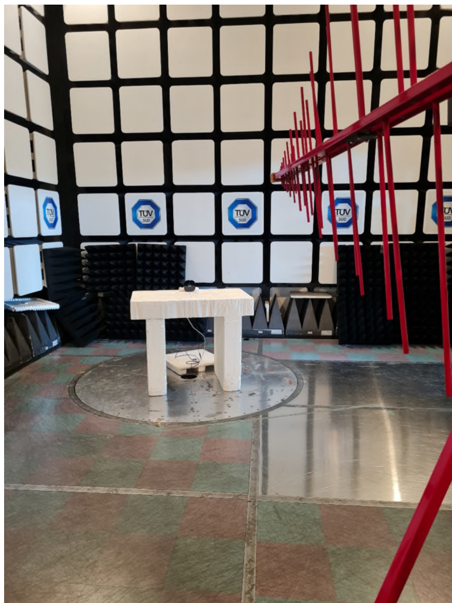
Figure 2 – Radiated Emissions Setup 30MHz – 1GHz
