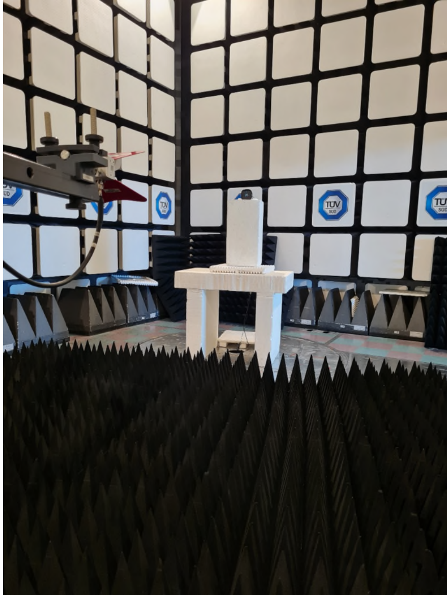
Figure 3 – Radiated Emissions Setup > 1GHz
