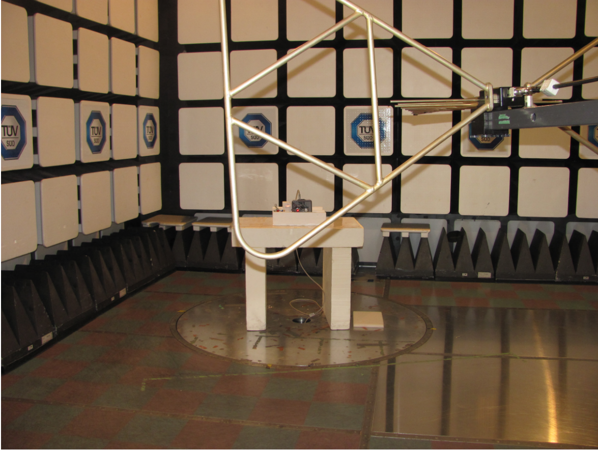
Figure 4 – Radiated Emissions Setup – Photo 3
