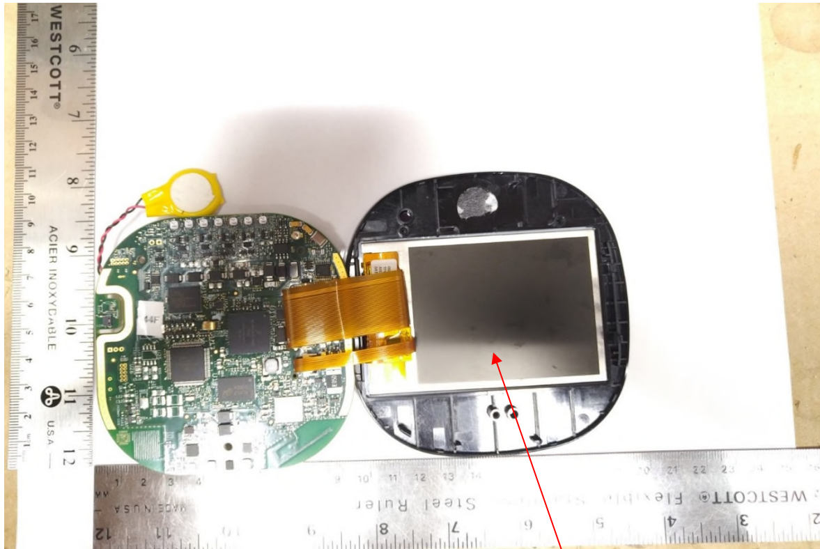
Figure 3 – EUT Internal View, PCB Front – Photo 1
