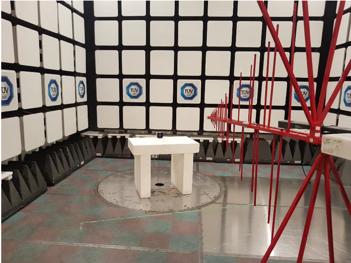
Figure 4 – Radiated Emissions Setup 30MHz – 1GHz
