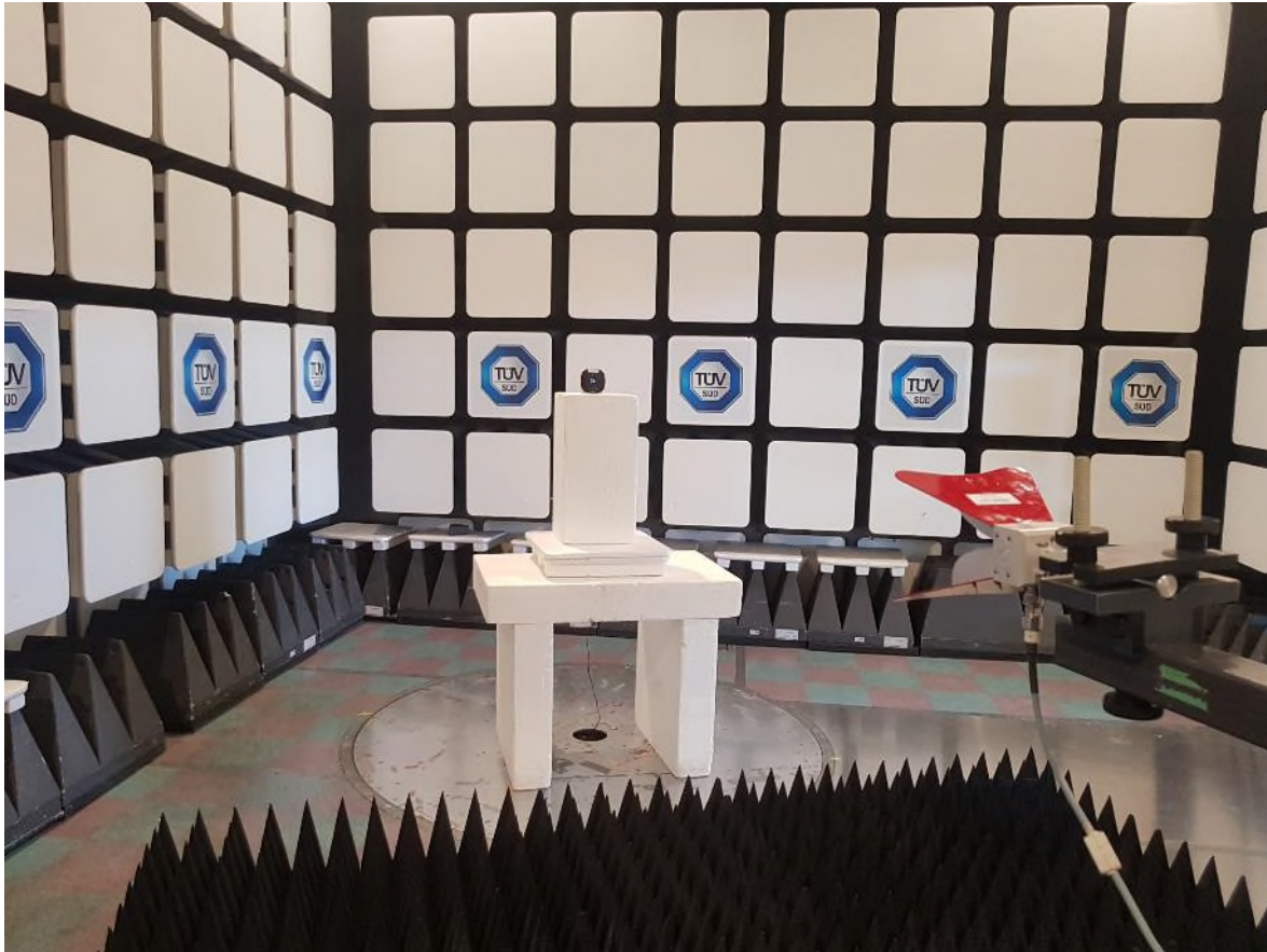
Figure 5 – Radiated Emissions Setup 1GHz – 18GHz
