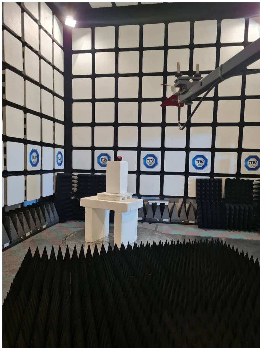
Figure 3 – Radiated Emissions Setup > 1GHz
