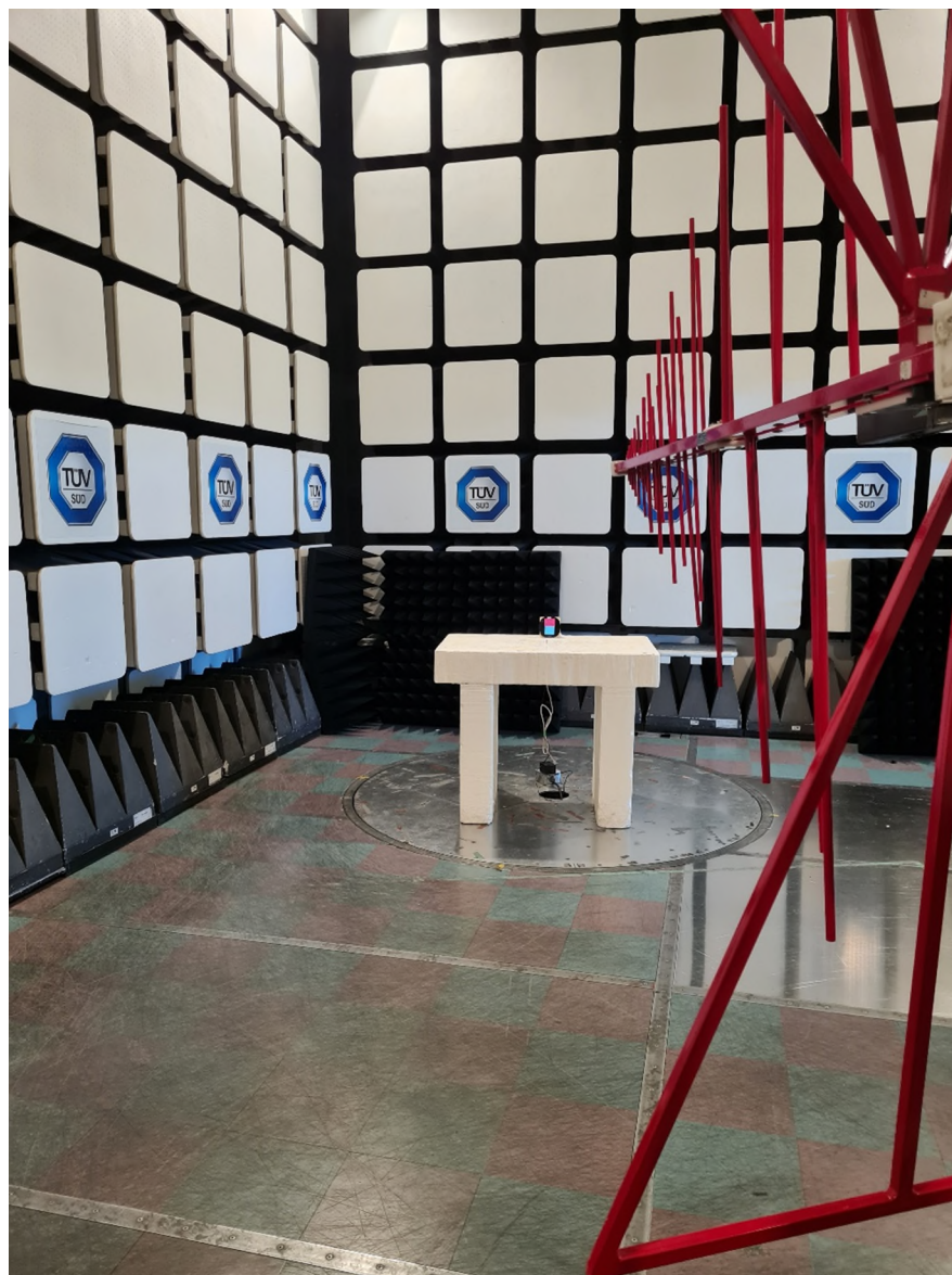
Figure 2 – Radiated Emissions Setup 30MHz – 1GHz
