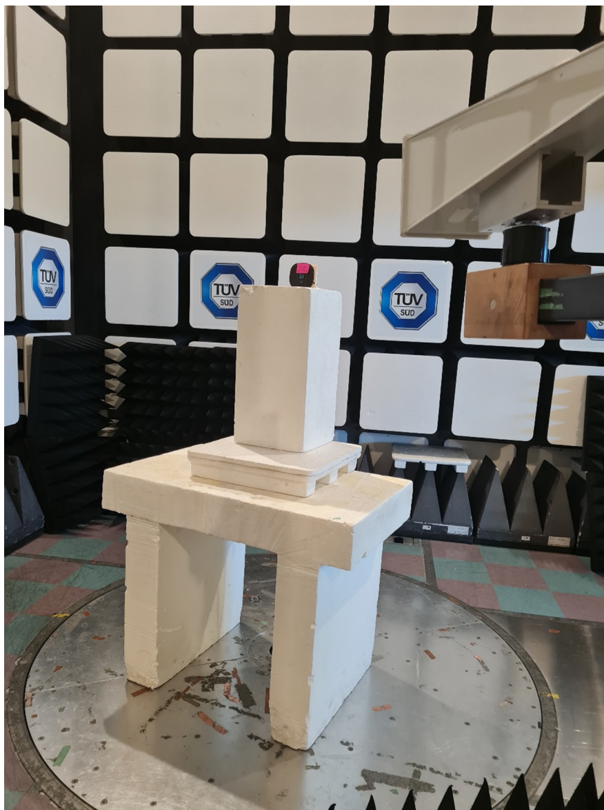
Figure 4 – Radiated Emissions Setup > 1GHz
