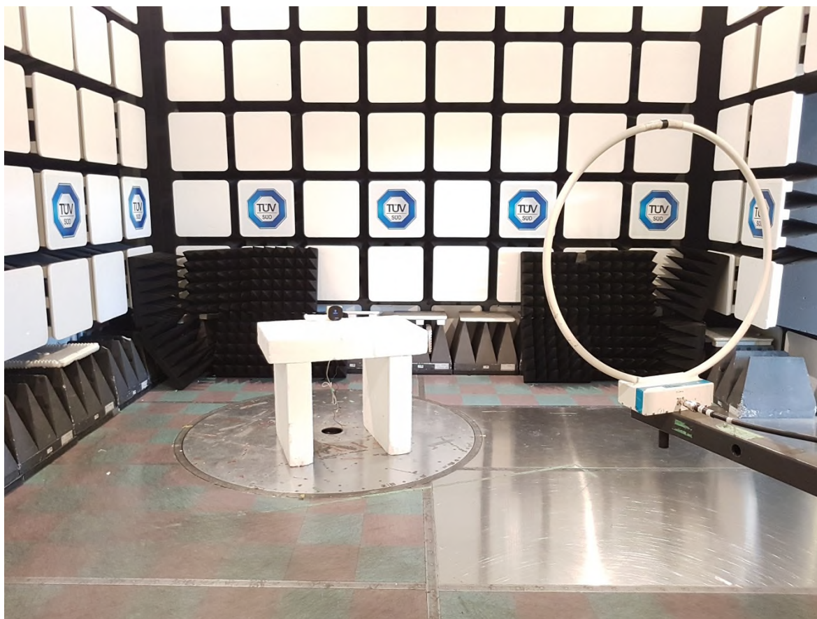
Figure 4 – Radiated Emissions Setup 9kHz – 30MHz
