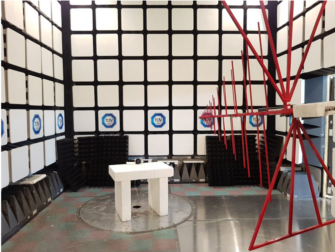
Figure 5 – Radiated Emissions Setup 30MHz – 1GHz
