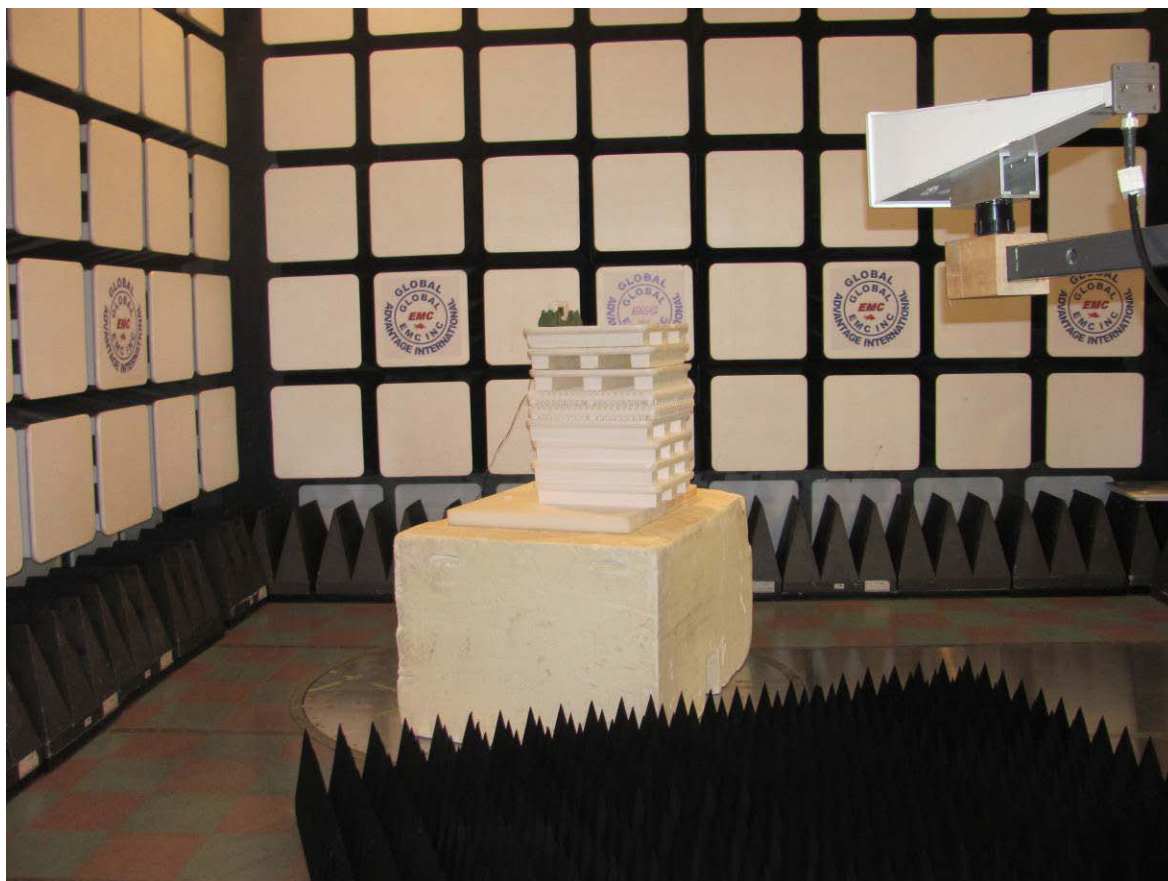
Figure 4: Radiated emission setup – photo 3
