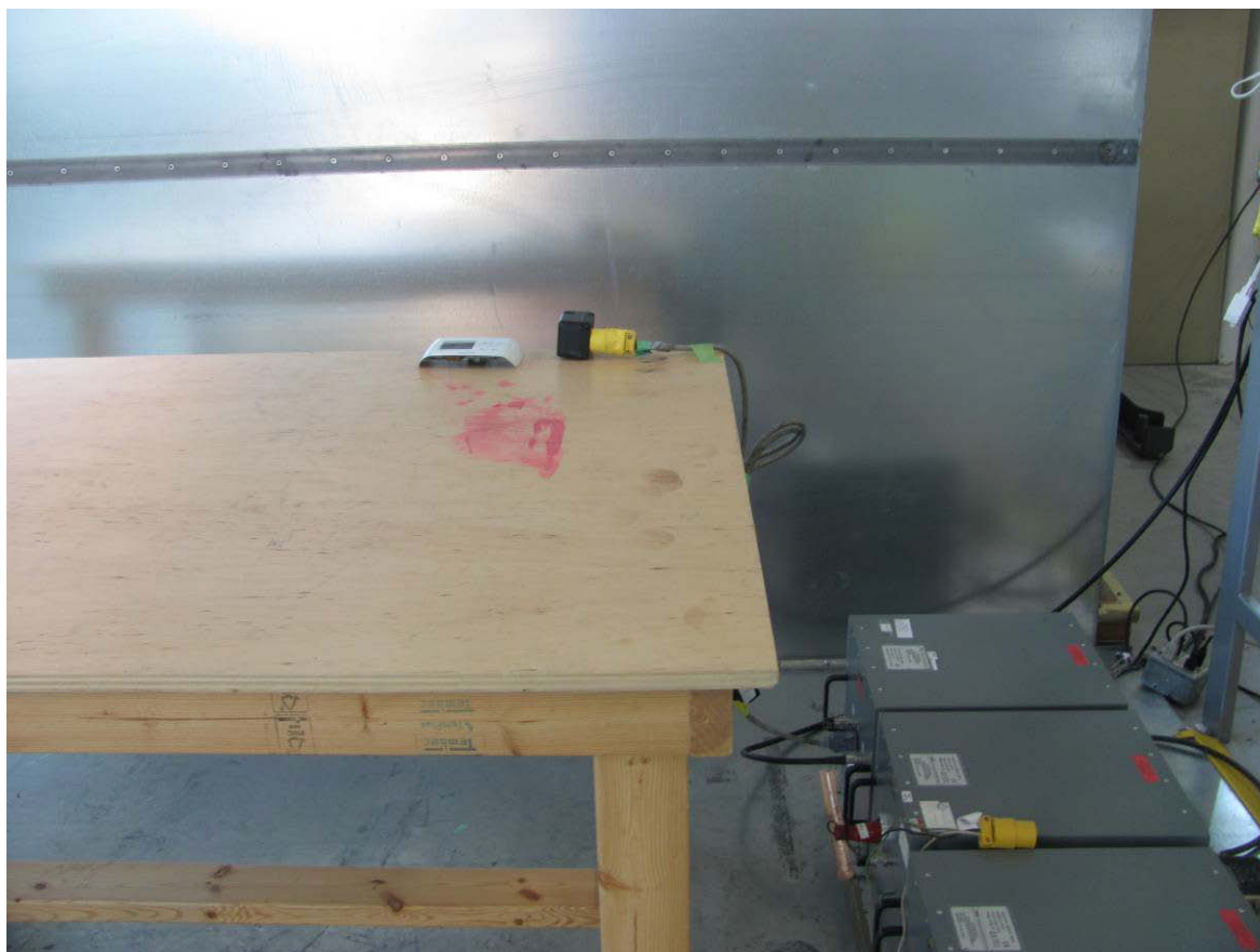
Figure 7: Power line conducted emission setup – photo 1
