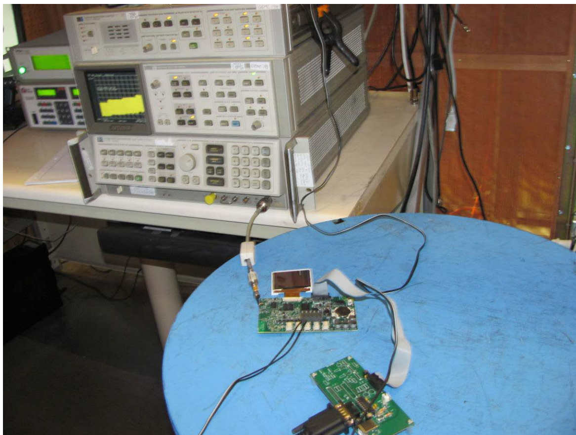
Figure 5: Antenna port conducted emission setup – photo
