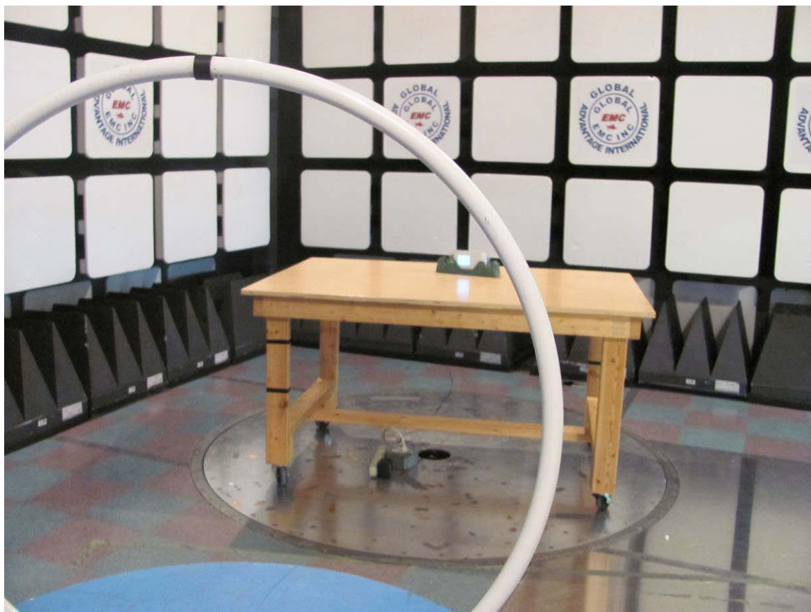
Figure 1: Radiated emission setup – photo 1
