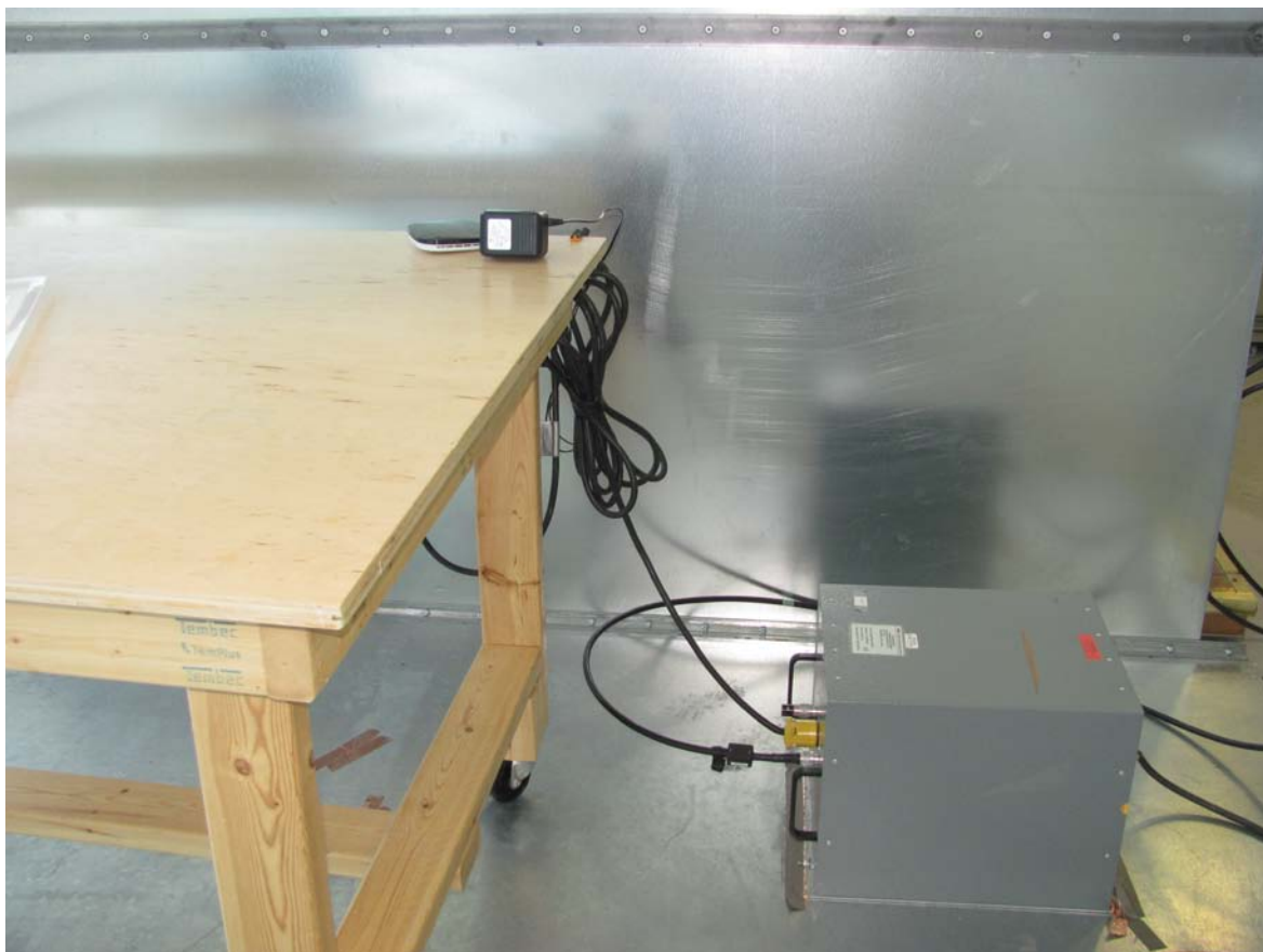
Illustration 7: Power line conducted emission setup – photo 1
