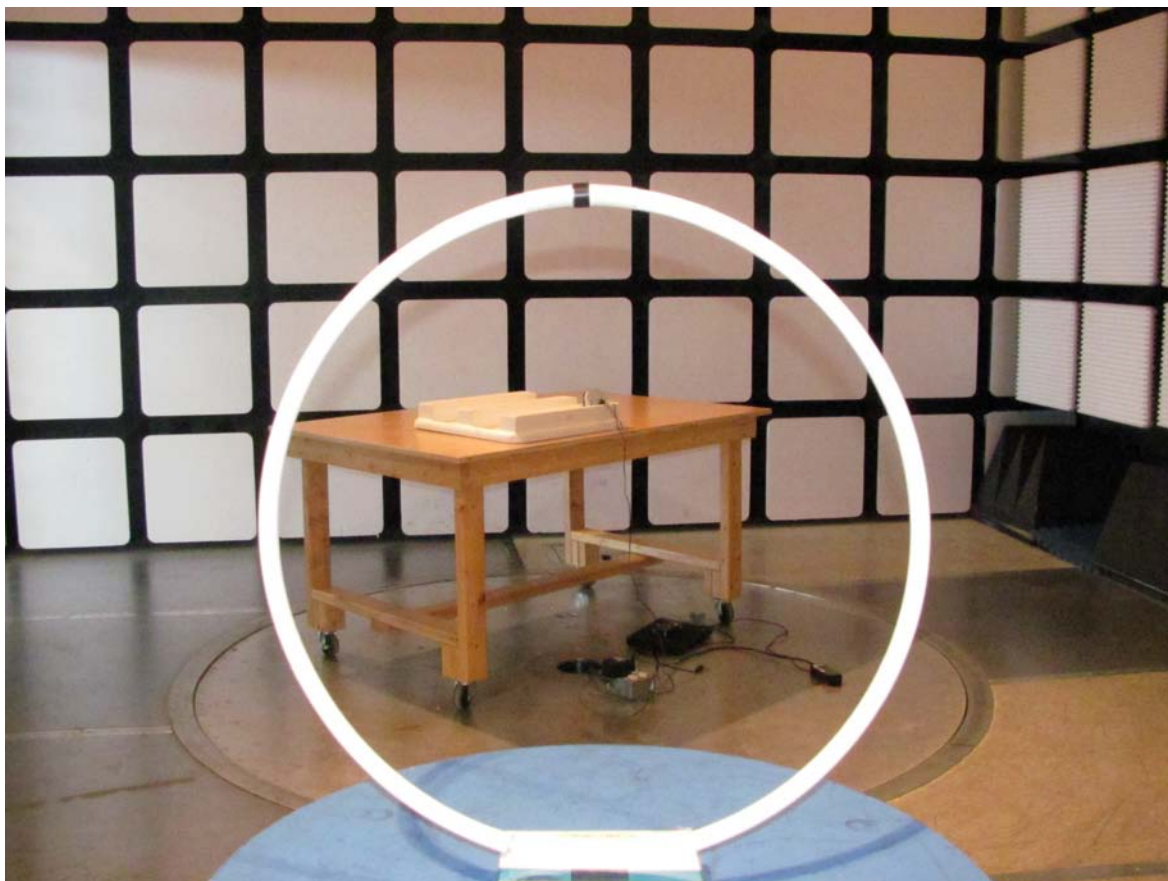
Illustration 3: Radiated emission setup – photo 1
