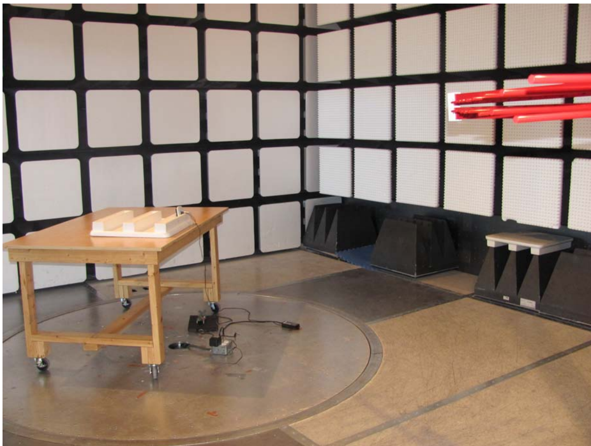
Illustration 4: Radiated emission setup - photo 2
