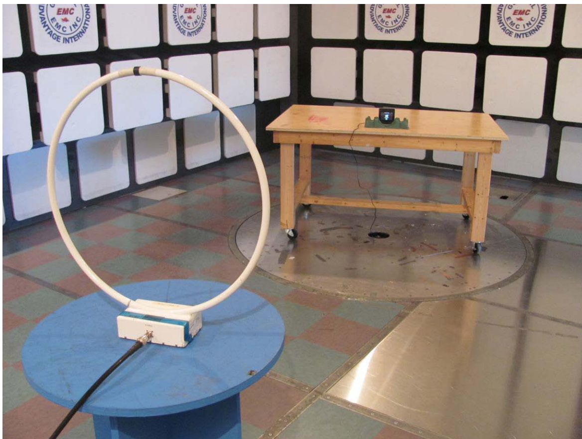
Figure 4: Radiated emission setup – photo 1
