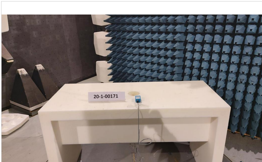
Photograph 1: EUT Test Setup in the Semi anechoic chamber, Radiated interference field
