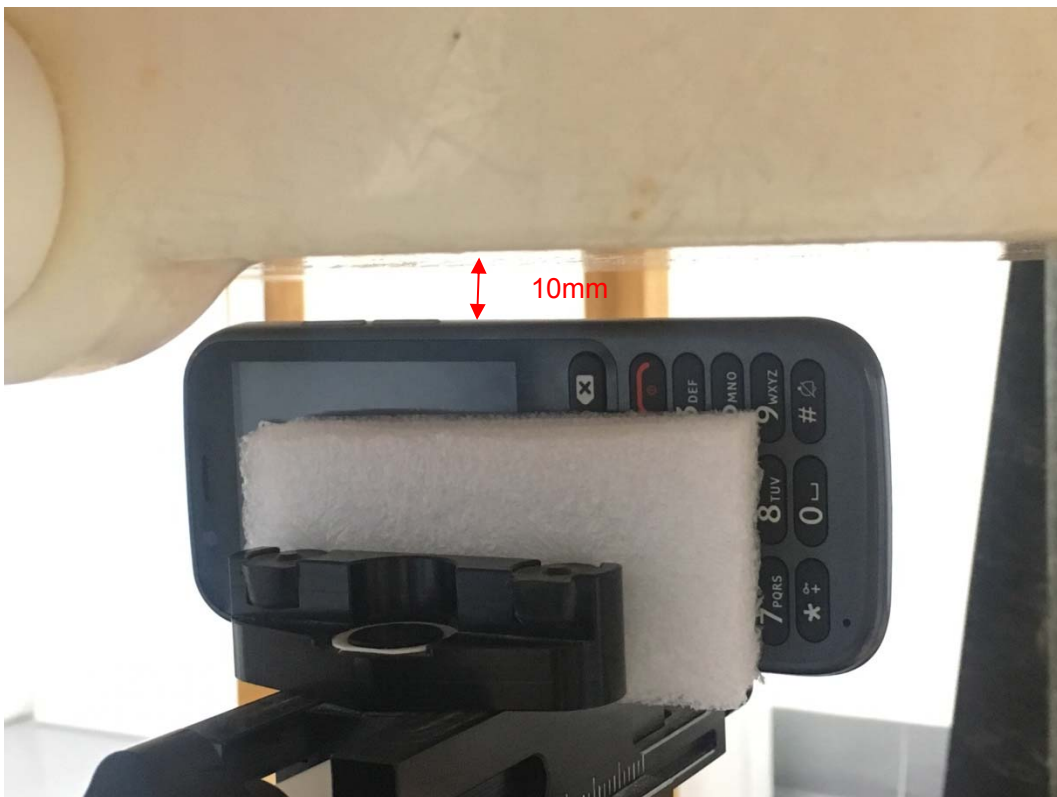
Picture 13: Right Side, the distance from handset to the bottom of the Phantom is 10mm
