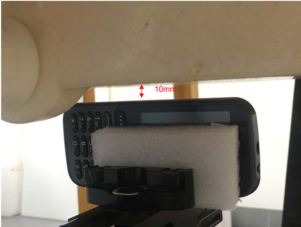
Picture 12: Left Side, the distance from handset to the bottom of the Phantom is 10mm
