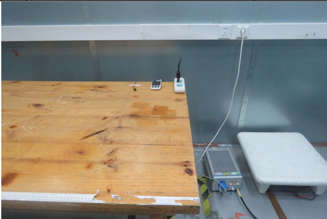
Picture 3 Conducted Emission Test Setup
