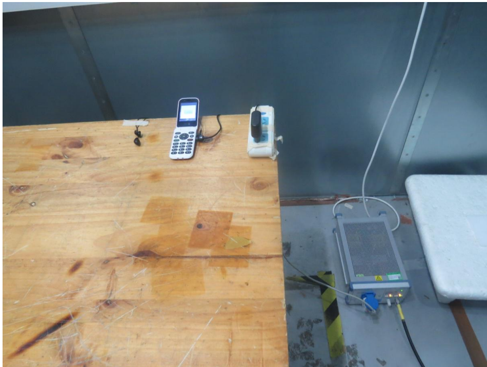
Picture 3 Conducted Emission Test Setup
