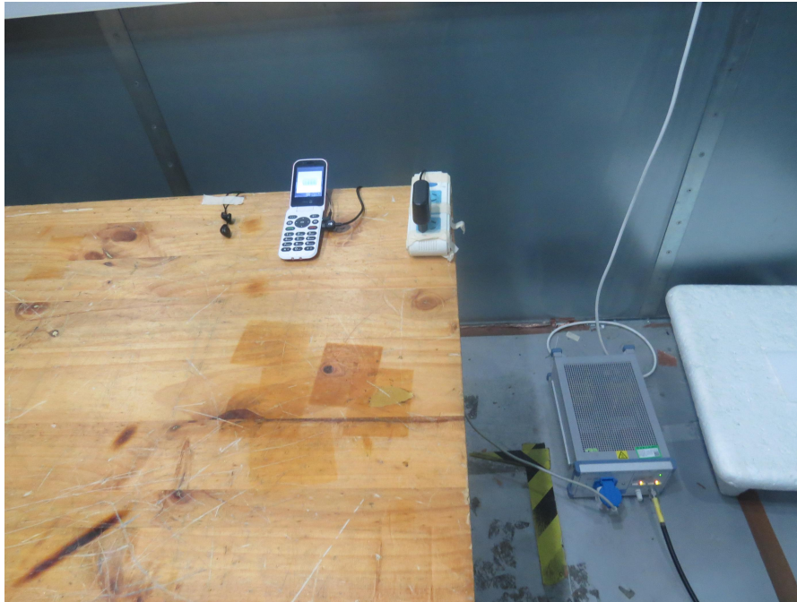
Picture 3 Conducted Emission Test Setup
