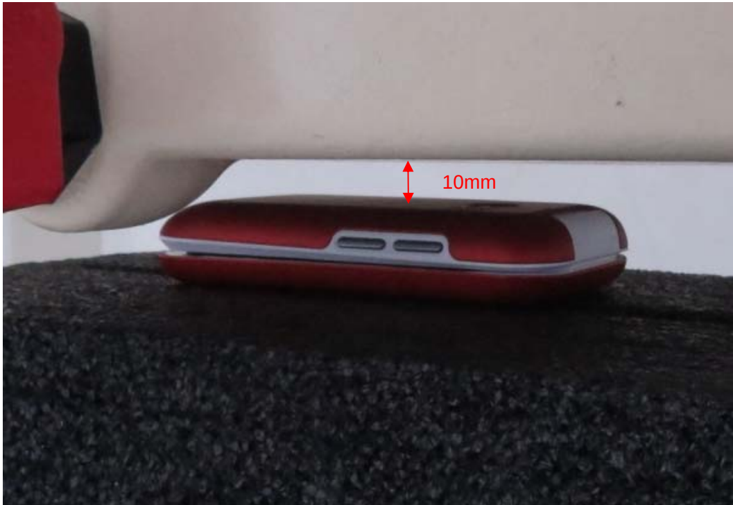
Picture 9: Back Side Close, the distance from handset to the bottom of the Phantom is 10mm
