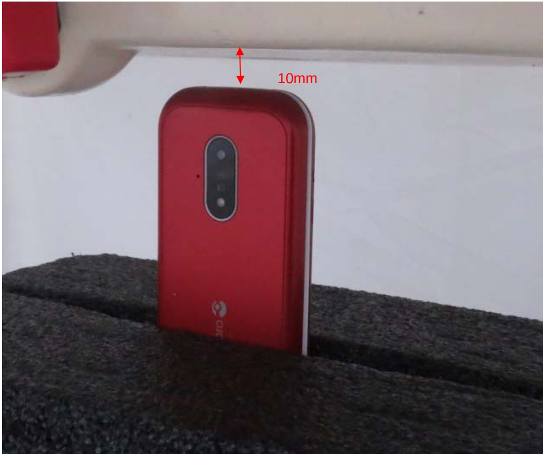
Picture 13: Top Side Close, the distance from handset to the bottom of the Phantom is 10mm
