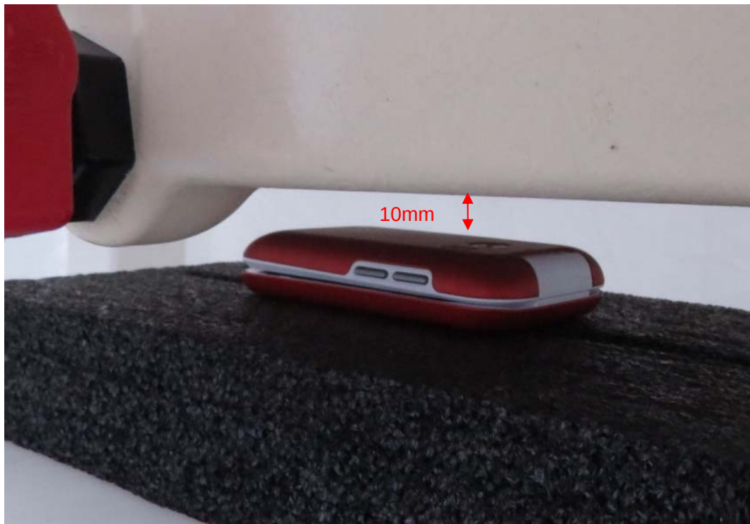
Picture 6: Back Side Close, the distance from handset to the bottom of the Phantom is 15mm
