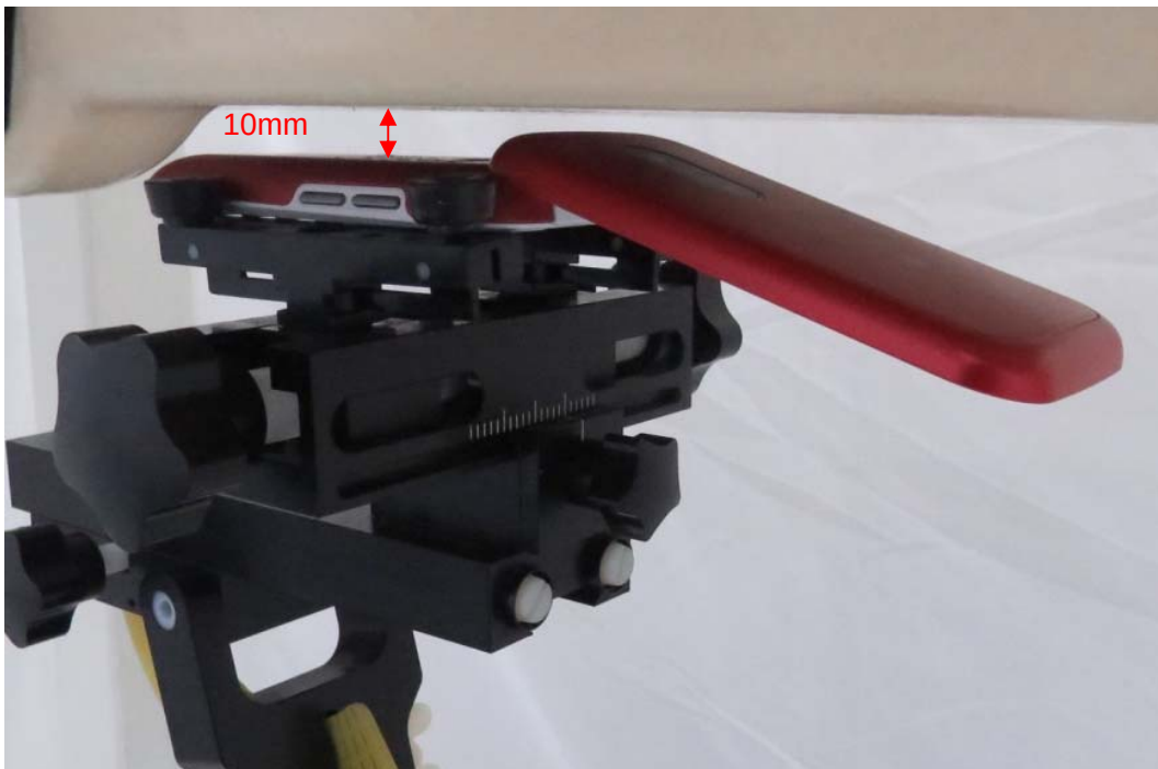
Picture 8: Back Side Open, the distance from handset to the bottom of the Phantom is 10mm
