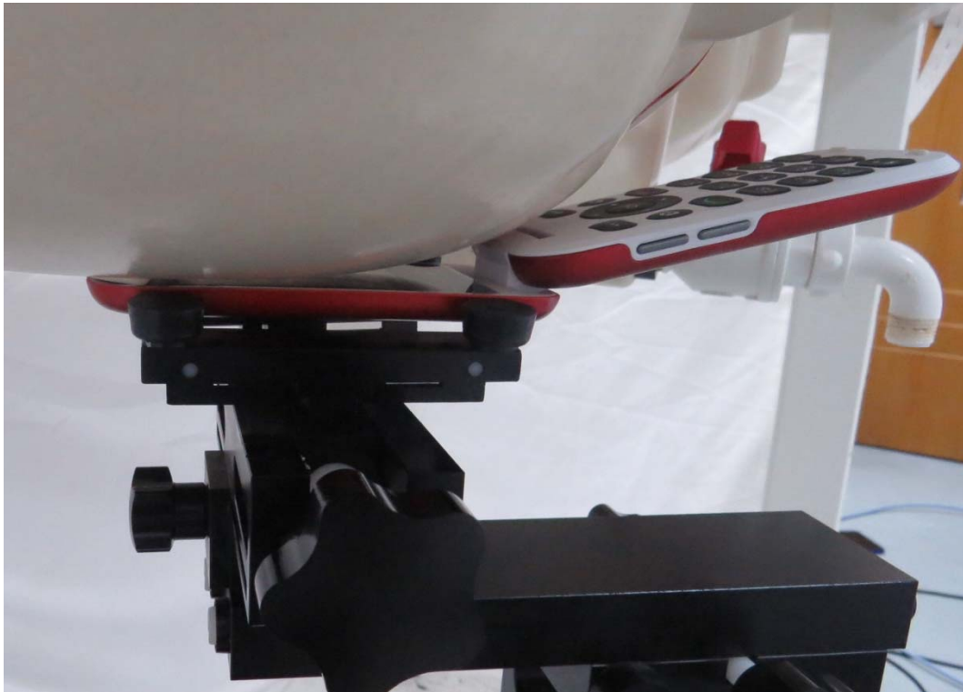
Picture 3: Right Hand Touch Cheek Position
