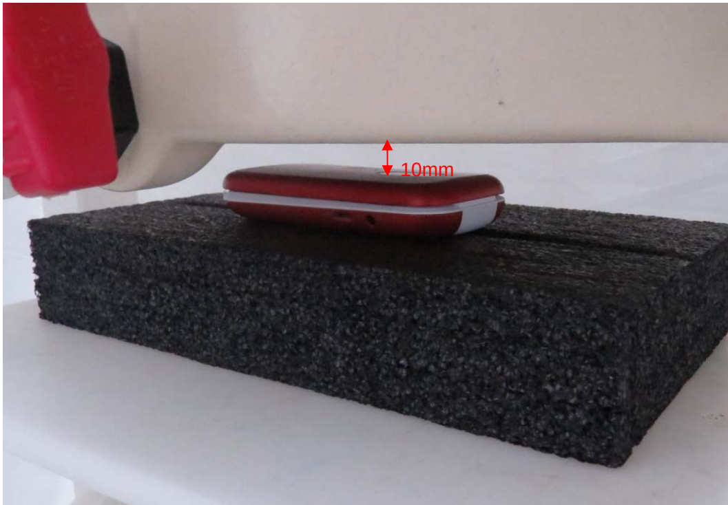
Picture 7: Front Side Close, the distance from handset to the bottom of the Phantom is 15mm
