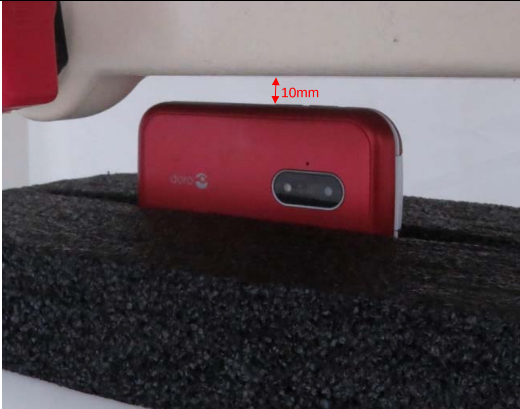
Picture 11: Left Side Close, the distance from handset to the bottom of the Phantom is 10mm
