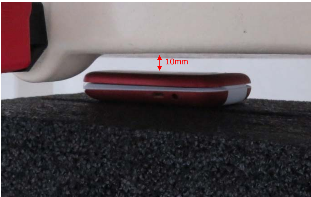
Picture 10: Front Side Close, the distance from handset to the bottom of the Phantom is 10mm
