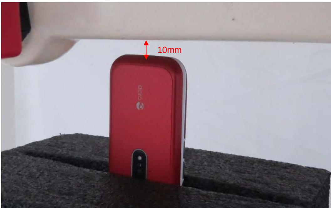
Picture 14: Bottom Side Close, the distance from handset to the bottom of the Phantom is 10mm
