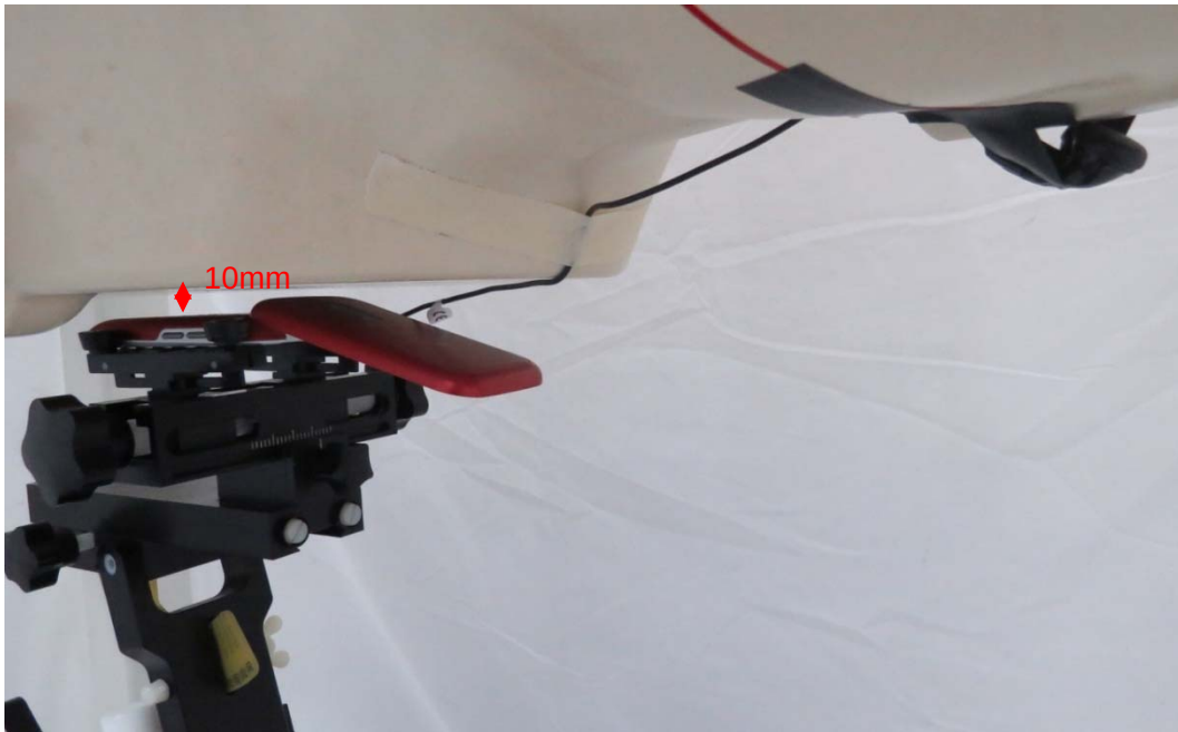
Picture 15: Back Side Open with Earphone, the distance from handset to the bottom of the Phantom is 10mm
