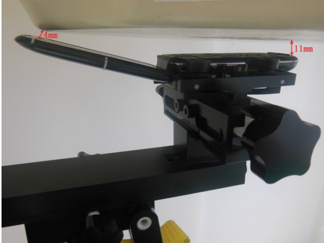
GSM1900 Right Cheek-SAR in mouth area(Flip Open)
