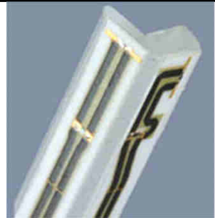
Fig 5.2 Photo of E-field Probe
