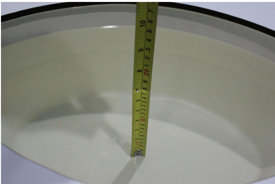
Picture 7-10: Liquid depth in the Flat Phantom (5G)
