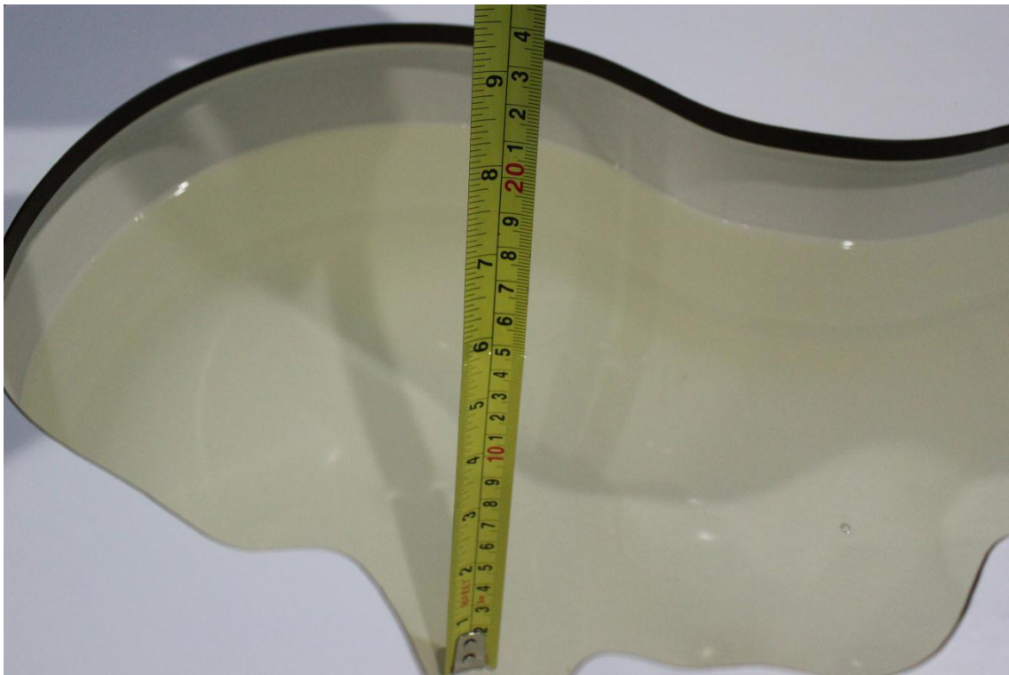
Picture 7-9: Liquid depth in the Head Phantom(5G)
