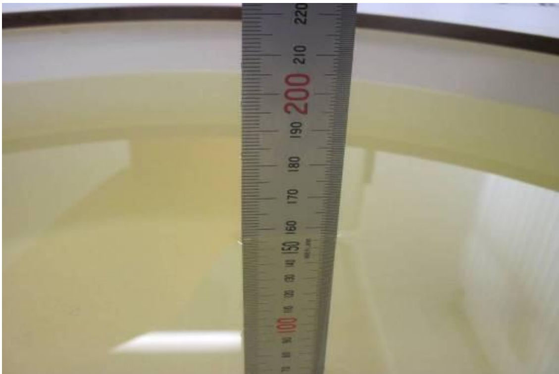
Picture 7-4: Liquid depth in the Flat Phantom (1900MHz)
