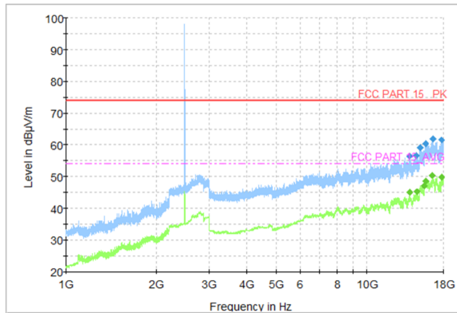
Fig. 72 Radiated Spurious Emission ( \pi/4 DQPSK, Ch78, 1 GHz ~18 GHz)
