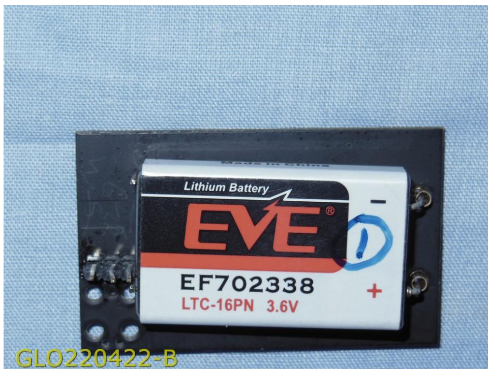
Internal View – PCB Rear With Battery Attached
