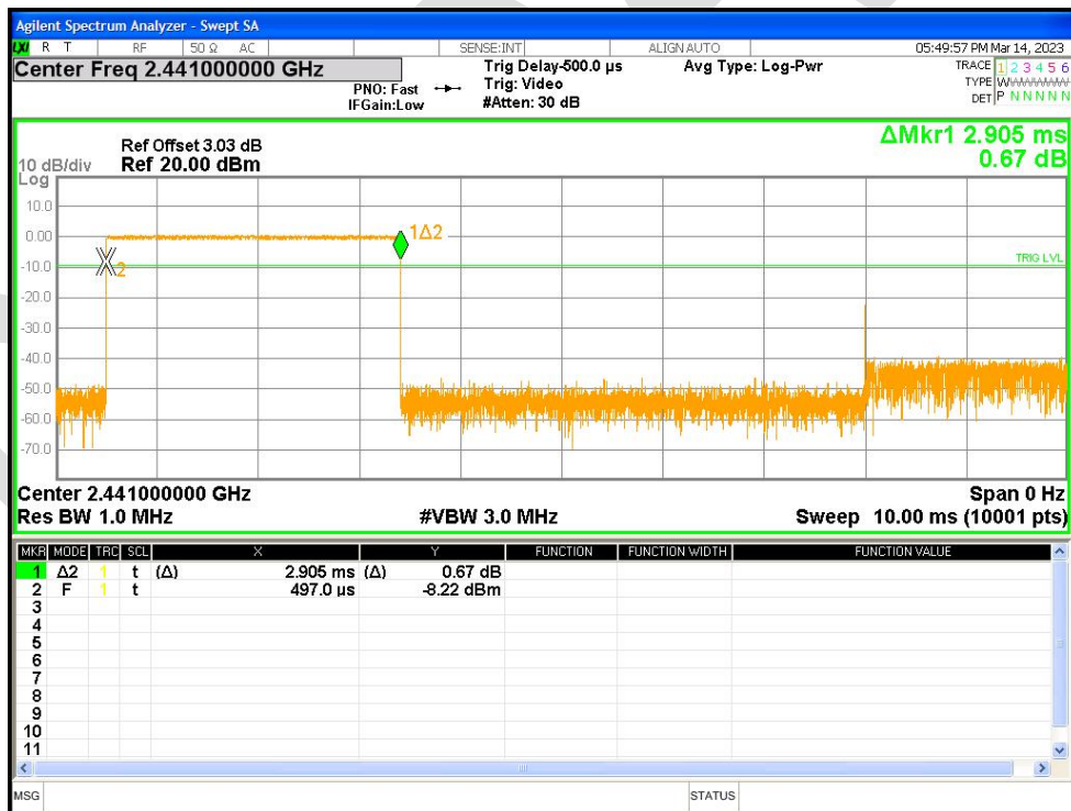
Dwell NVHT 1-DH5 2441MHz Ant1 Accumulated
