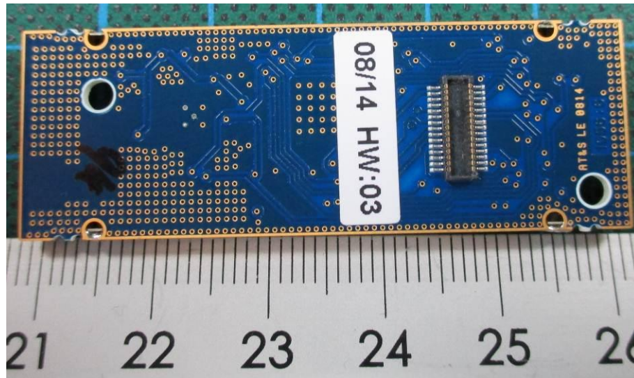
145725_44.JPG: RF Module 1 – Bottom View
